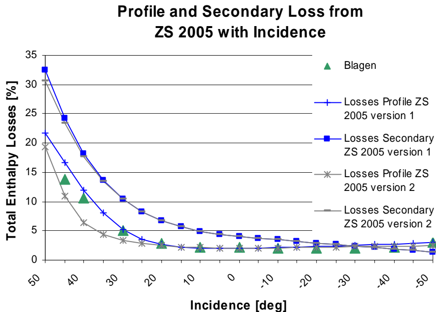
Figure 4.3-18: Comparison between ZS 2005 Version 1 and Version 2 profile and secondary losses with the profile losses from Blagen. Both versions are “no limit”.
