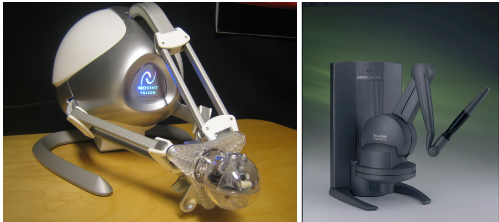
(a) The Falcon, developed by Novint, is a commercial force-reflecting joystick[51]
