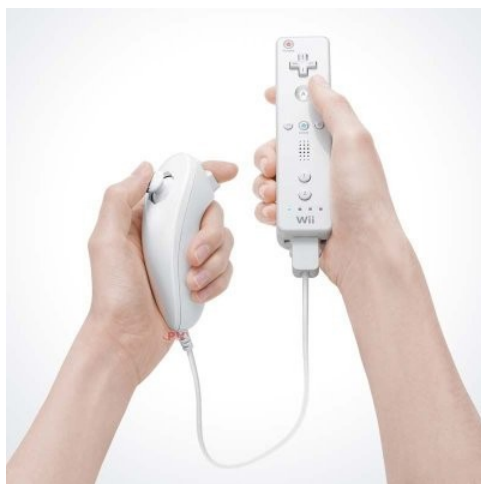
Figure 5.4: Nintendo Wii Remote (on the right) and Nunchuck (on the left) controllers
