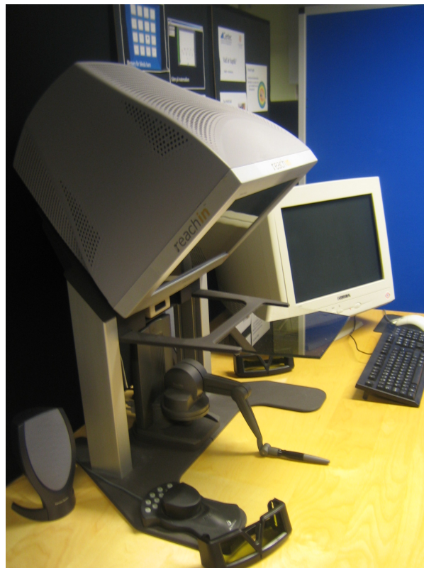
Figure 2.12: Pen-based force-feedback ground-referenced device located at the Virtual Reality lab, IKDC, Lunds Universitet
