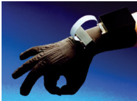
Figure 2.8: A bend-sensing data glove
