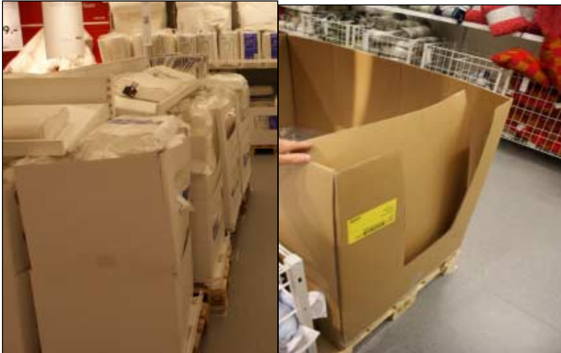
Figure 4:4 A and B Failures in RSP designs
