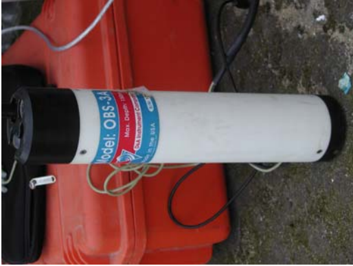
Figure 32 Picture of OBS-3A WSE measuring instrument utilized at field station S01
