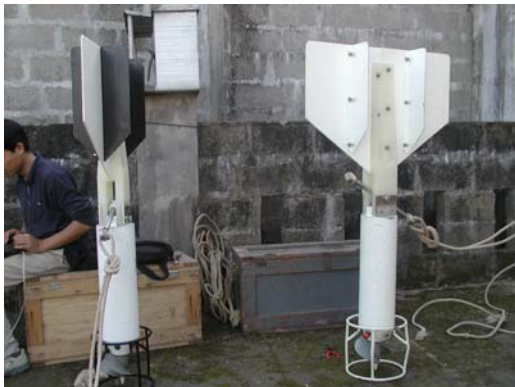
Figure 31 Picture of DNC-2M current measuring instruments utilized at field stations S01 and S02
