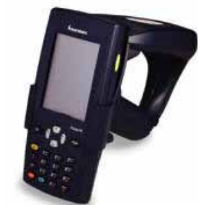
Figure 9 IP3 Intellitag portable reader [24]
