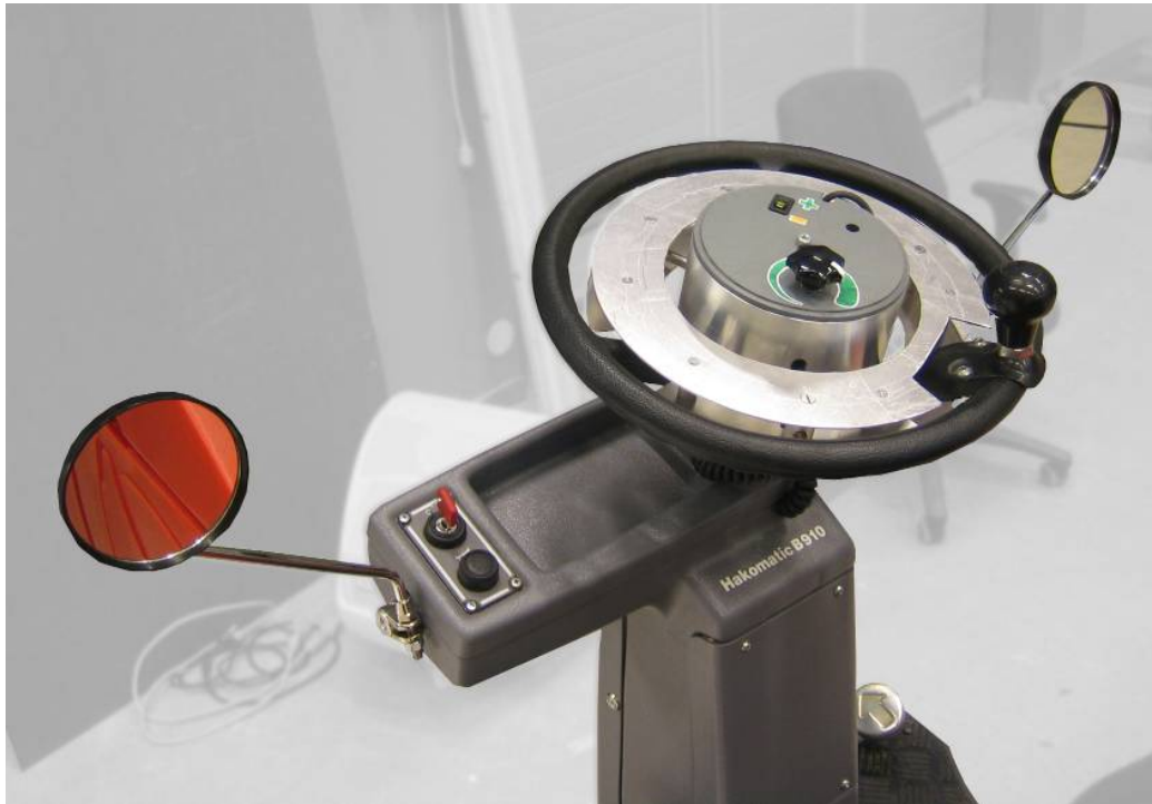
Prototype with hand controlled accelerator, speed and reverse controls
