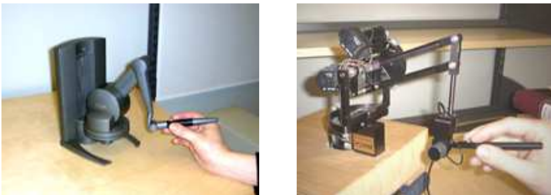
Figure 2.1 The Phantom haptic device. The left picture shows the Phantom desktop model and the right picture shows the Phantom Premium 1.0 model.
