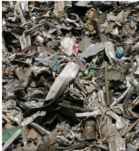
Figure 3-5 Heavy fraction of shredder residue (2)
