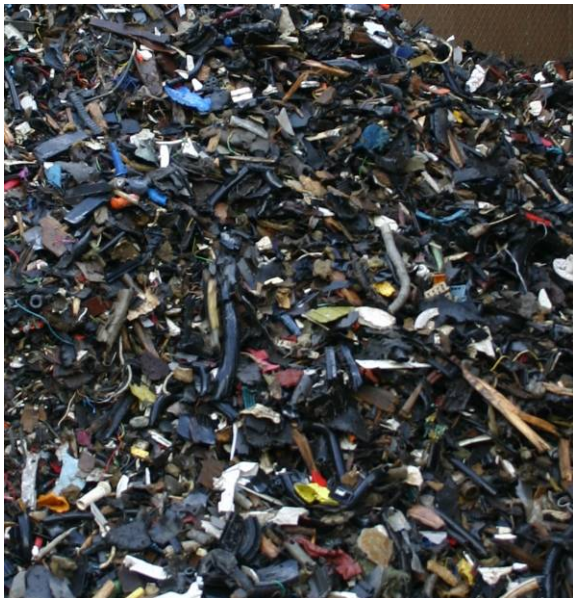
Figure 3-4 Heavy fraction of shredder residue (1)
