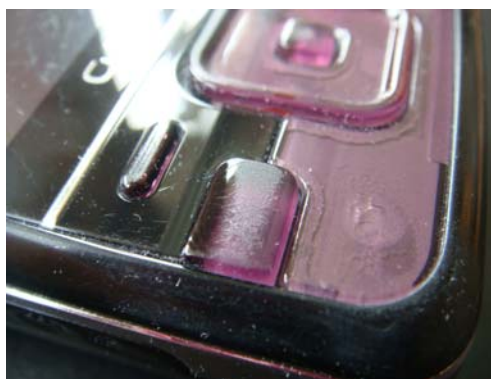
Result of the abrasion tumbling test
