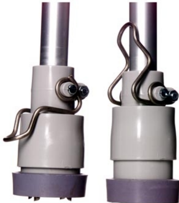
Figure 25. Ice pick with 4 spikes is a complete ice pick with built-in spikes easy to fold in and out with the foot or the hand. Plastic inserts are included for adjustment to the most frequent tube diameters. ("Swereco")
