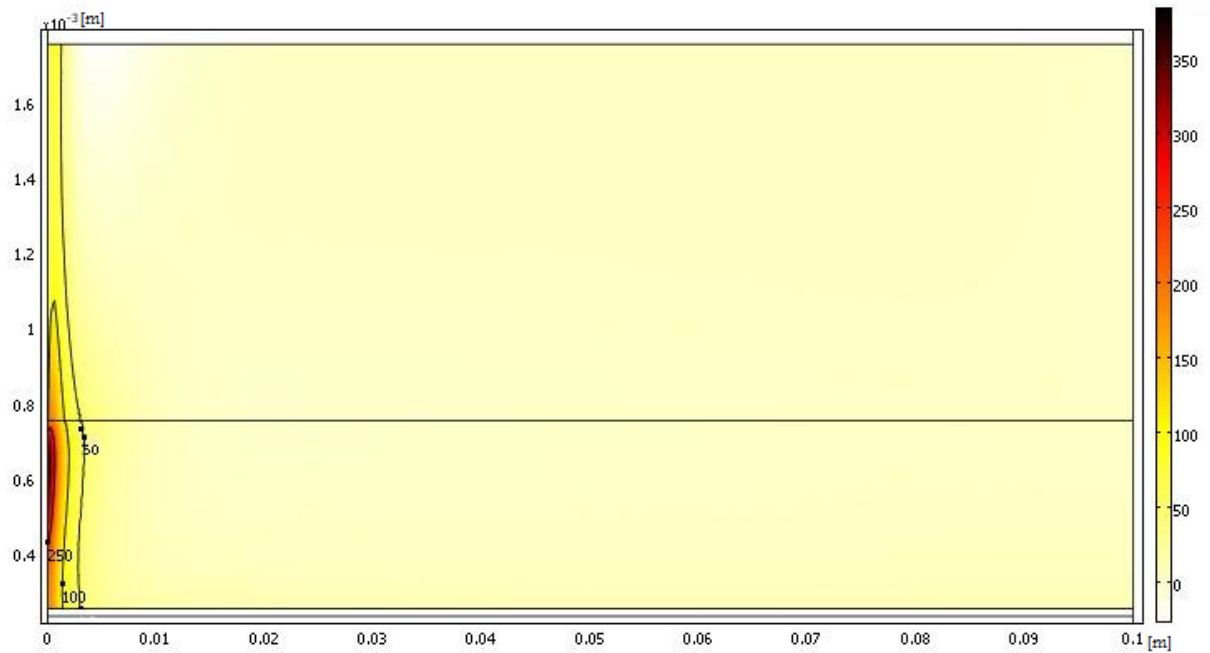
Figure 13: The reaction rate for the water-gas shift reaction [\text{mol}/(\text{s}\cdot\text{m}^3)] in the anode and fuel channels for Achenbach & Riensche's model.
