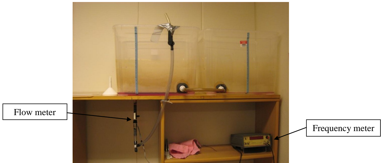
Figure 27 Flow meter and tanks for saline water used in the experiment
