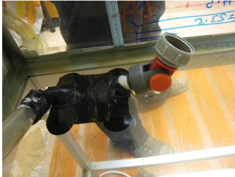
Figure 29 Nozzle support system on which the nozzle was attached
