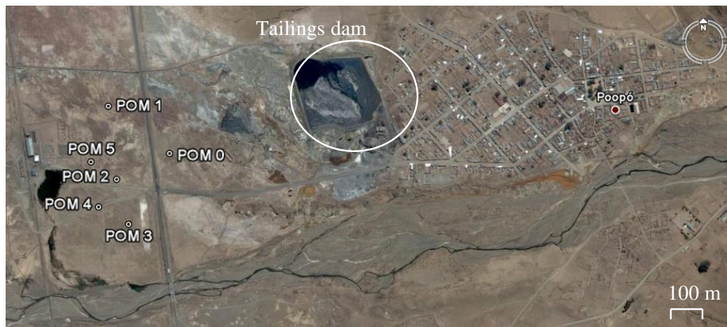
Figure 4-5. Piezometers POM 0-5 downstream the tailings dam (dark blue in the center) just west of the village Poopó (Google Earth, 2009).
