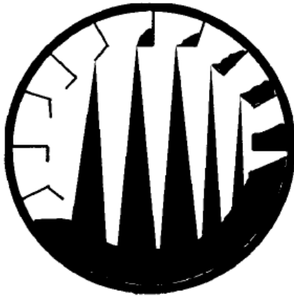
Figure 2-12. Typical flight arrangement in a direct rotary dryer [23].
