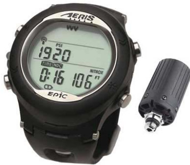
Wrist watch dive computer. In this case air integrated, so that it also monitors remaining air. The plug to the right is a pressure gauge and a wireless transmitter mounted on the first stage.
