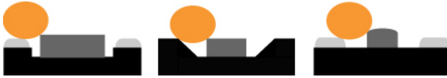
Figure 11.1. Cross-section of three mobile phones which illustrates the space when grasping the joystick. Left: SE K700, Middle: SE K750, Right: SE W800.
