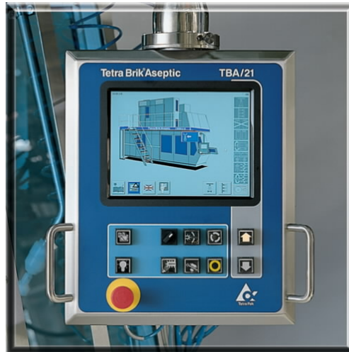
Figure 2. The TPOP consists of a touch screen and a set of hardware buttons.
