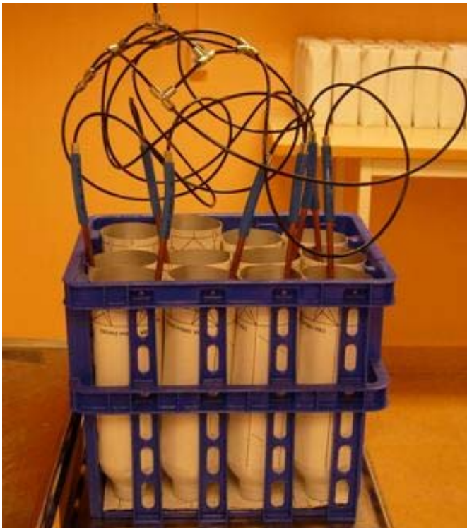
Figure 19 shows the set up when eight packages had their dissolved oxygen removed.
