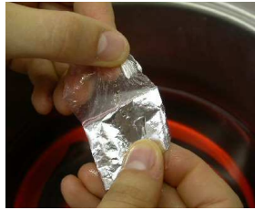
Figure 43: Removal of inside layer and adhesion test
