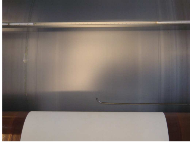
Figure 40: The sniffer with the bent end placed in the middle of the web
