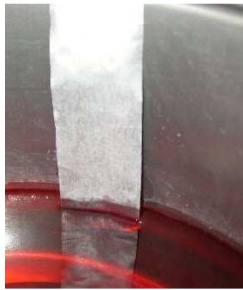
Figure 43: Removal of inside layer and adhesion test
