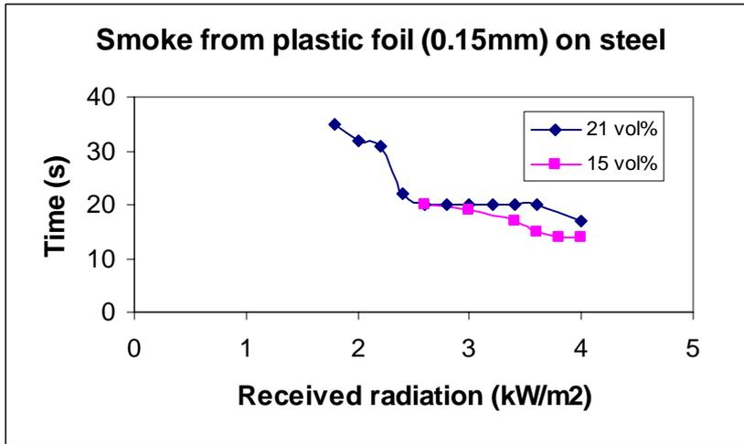
Figure H.7 Time to emit smoke at different radiation levels and oxygen concentrations.
