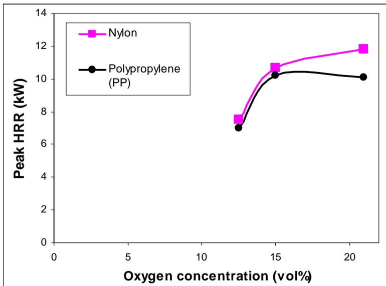
Figure 4.14 Peak HRR (kW) of nylon and polypropylene (PP) in different oxygen concentration (vol%). Data is measured with a cone calorimeter with external radiation of  $50\text{kW/m}^2$  and gas inflow of  $180\text{ l/min}$  [17].
