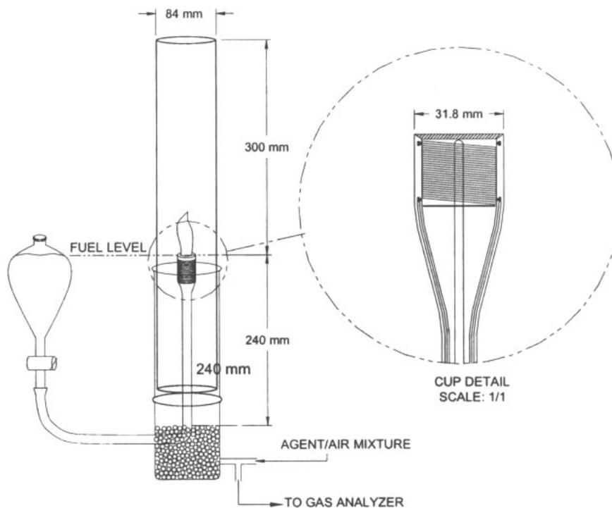
Figure E.1 Apparatus for cup burner suited for class B materials [57].
