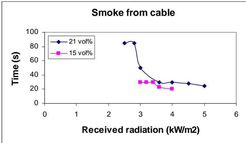
Figure 4.16 Time to emit smoke from cable at different radiation and oxygen concentration.
