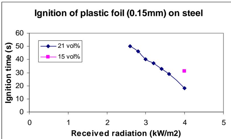
Figure H.2 Time to ignition at different radiation and oxygen concentrations.
