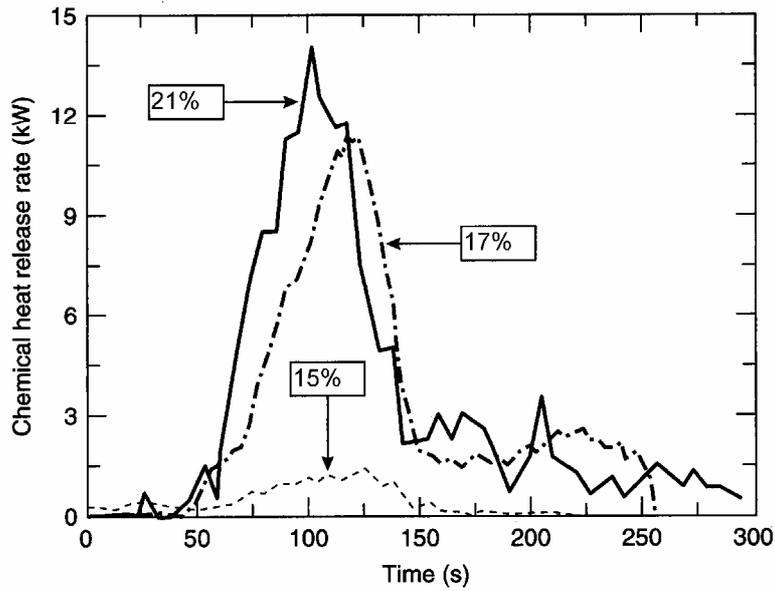
Figure 4.13 Heat release rate (kW) for burning paper boxes in 21, 17 and 15 vol% oxygen without external radiation [26].
