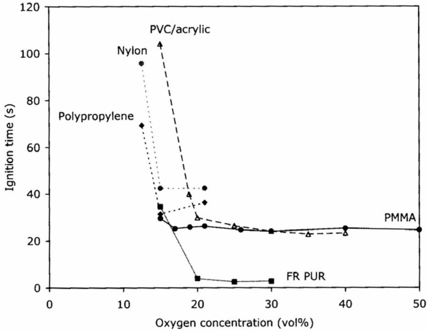
Figure 4.7 Ignition time (s) of different plastic materials in different oxygen concentrations (vol%). Heat flux is  $50\text{kW/m}^2$  [16].
