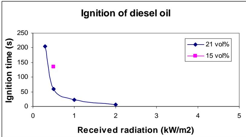
Figure H.4 Time to ignition at different radiation levels and oxygen concentrations.
