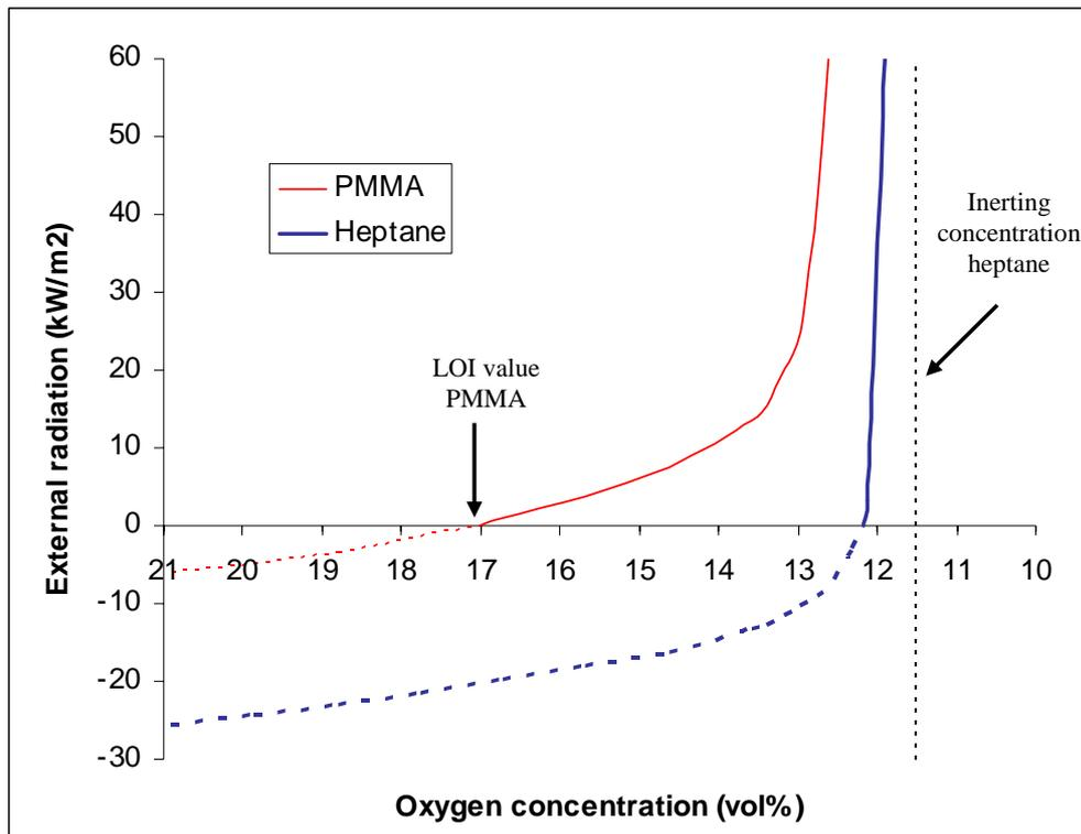
Figure 4.6 Oxygen concentration needed to extinguish a fire calculated by using the Fire point theory.
