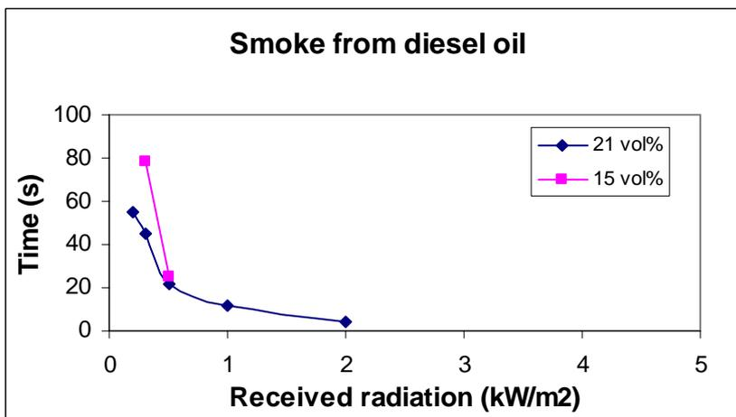
Figure H.9 Time to emit smoke at different radiation levels and oxygen concentrations.
