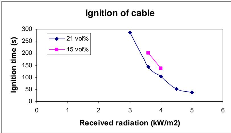
Figure 4.15 Time to ignition at different radiation levels and oxygen concentrations.
