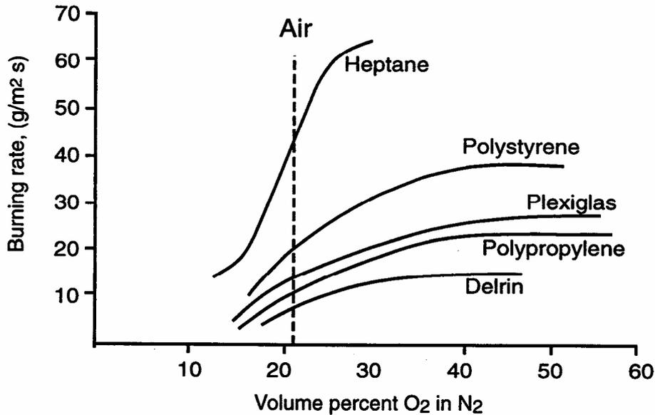
Figure 4.2 Burning rate of different class A and B materials in different oxygen concentrations [9].
