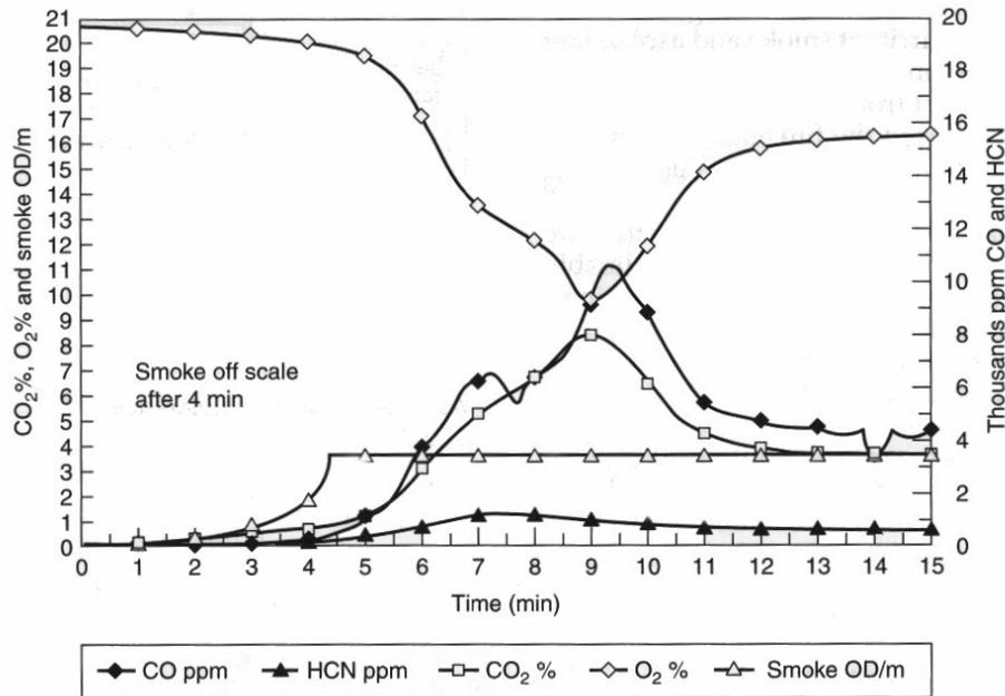
Figure 4.12 Gases and smoke analysis in full scale tests in an enclosure that starts with smouldering combustion [26].
