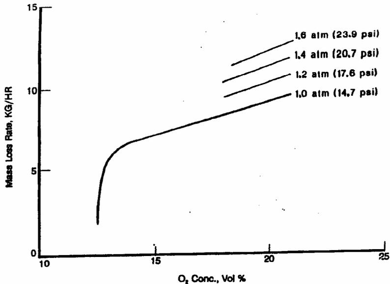
Figure 4.5 Experiments show the dependence of oxygen concentration and the small dependence of oxygen pressure on mass loss rate of a class B material (methyl alcohol) [8].
