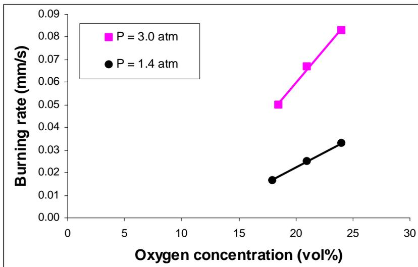
Figure 4.4 Experiments show the dependence of oxygen concentration on burning rate of class B material (Kerosene) [8].
