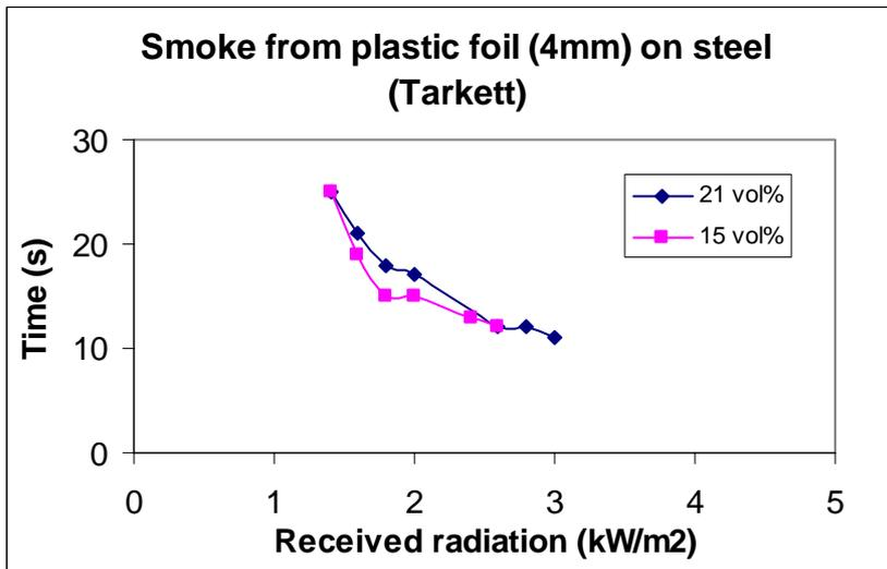
Figure H.8 Time to emit smoke at different radiation levels and oxygen concentrations.
