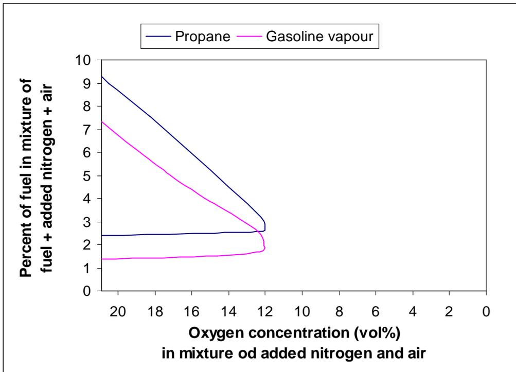
Figure F.3 Flammability limits and inerting concentration for propane and gasoline vapour.
