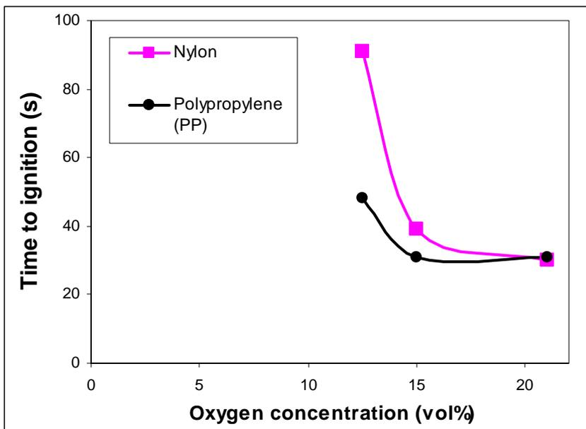
Figure 4.8 Ignition time (s) of nylon and polypropylene (PP) in different oxygen concentrations (vol%). Data is measured with a cone calorimeter with heat flux of  $50\text{kW/m}^2$  [17].
