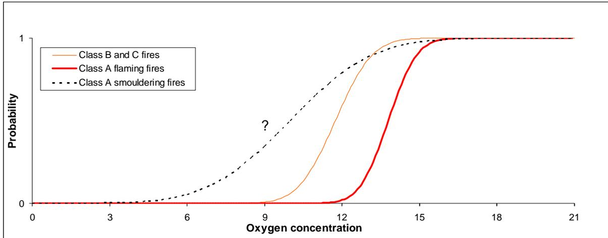
Figure 4.18 Probability that fire prevention fails in different oxygen concentrations. The probability of a fire is illustrated for different classes of materials.
