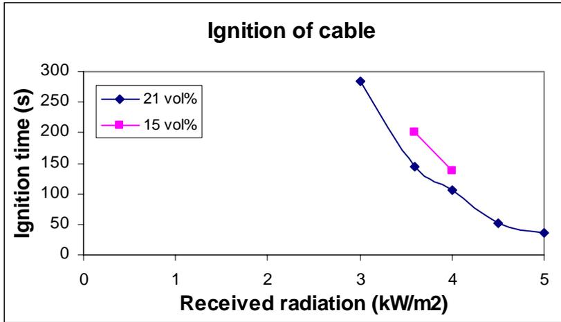
Figure H.1 Time to ignition at different radiation levels and oxygen concentrations.
