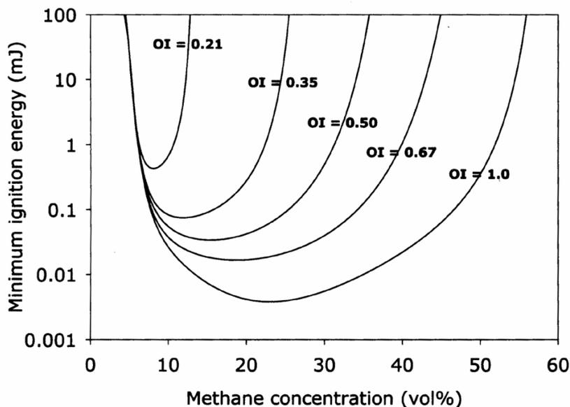
Figure 4.10 Minimum ignition energy (MIE) for methane in different oxygen concentrations [16]. OI is the oxygen concentration in volume fraction.
