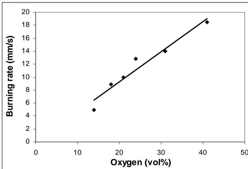
Figure 4.1 Burning rate of paper in different oxygen concentrations [8].
