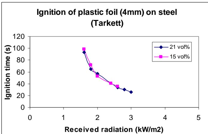
Figure H.3 Time to ignition at different radiation levels and oxygen concentrations.
