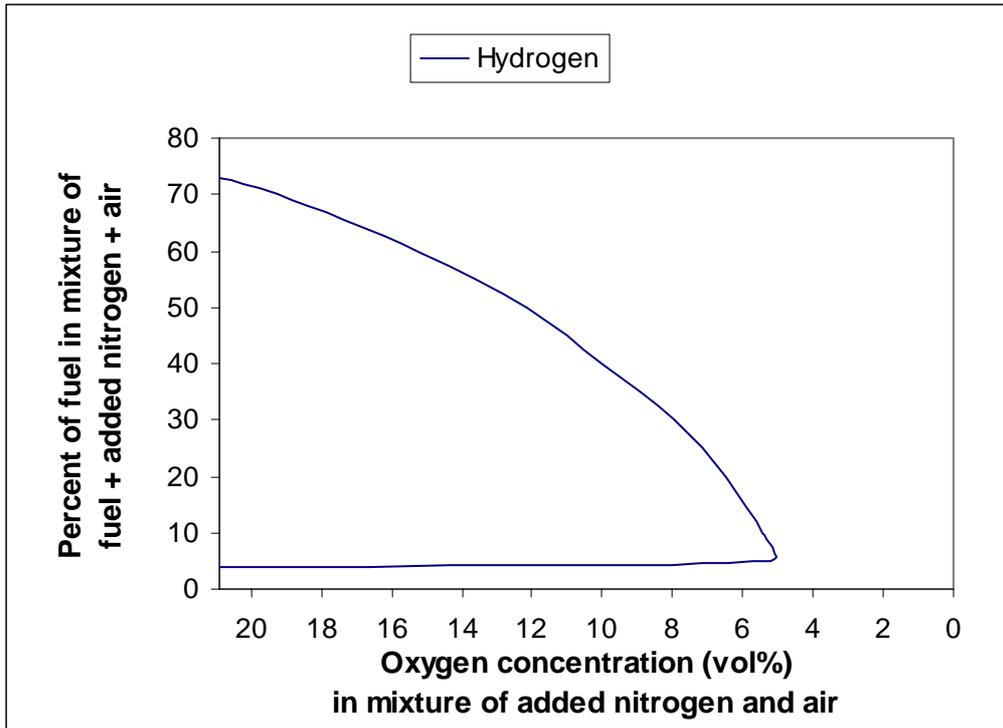
Figure F.2 Flammability limits and inerting concentration for hydrogen.
