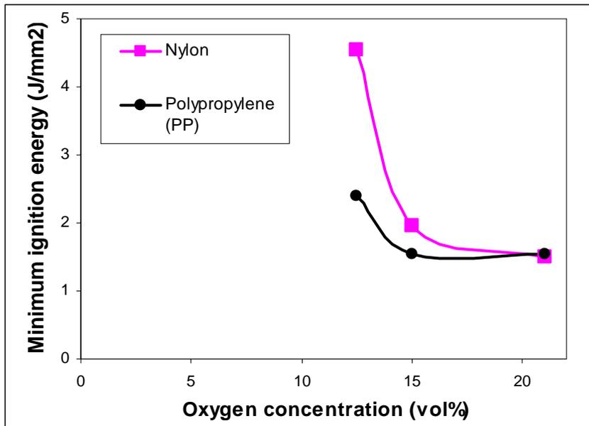
Figure 4.9 Minimum ignition energy (MIE) for class A materials in different oxygen concentrations [17].
