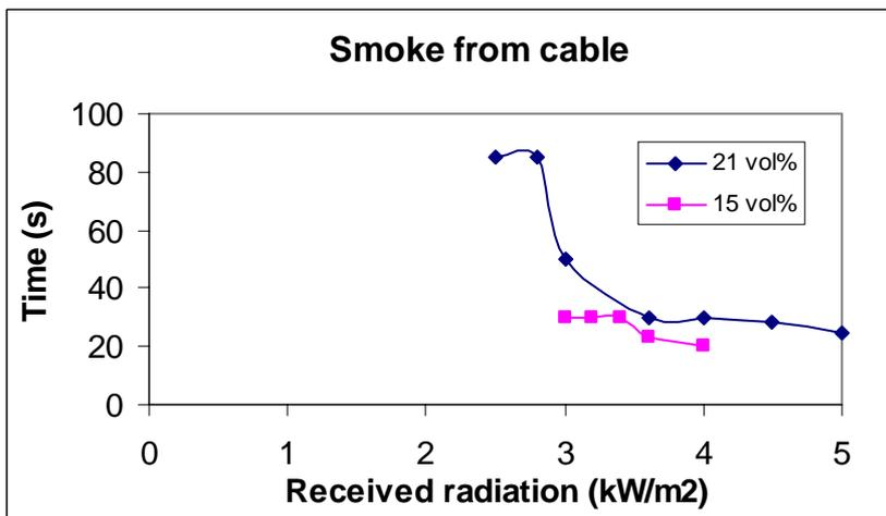
Figure H.6 Time to emit smoke at different radiation levels and oxygen concentrations.
