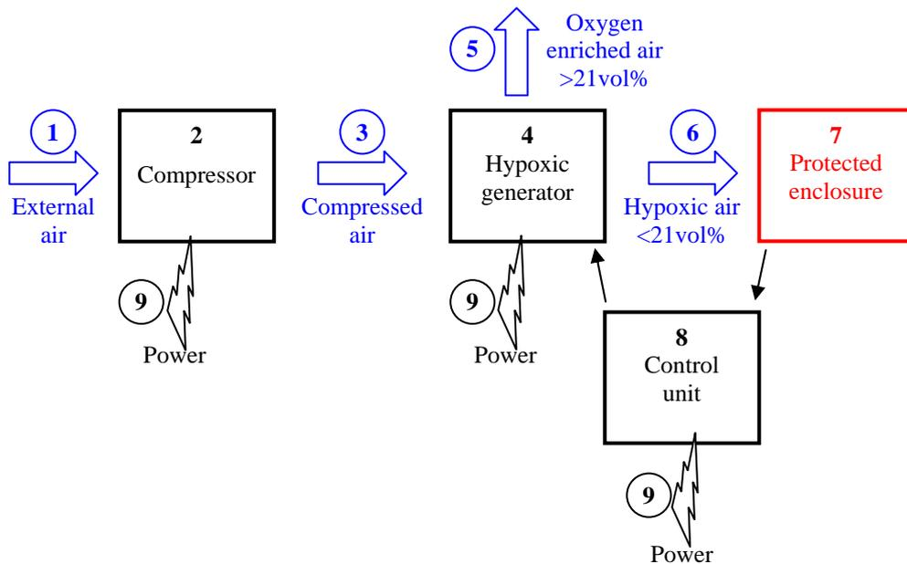
Figure 7.1 Typical concept of a hypoxic environment.
