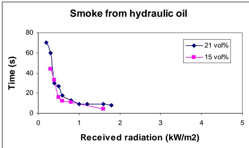
Figure H.10 Time to emit smoke at different radiation levels and oxygen concentrations.
