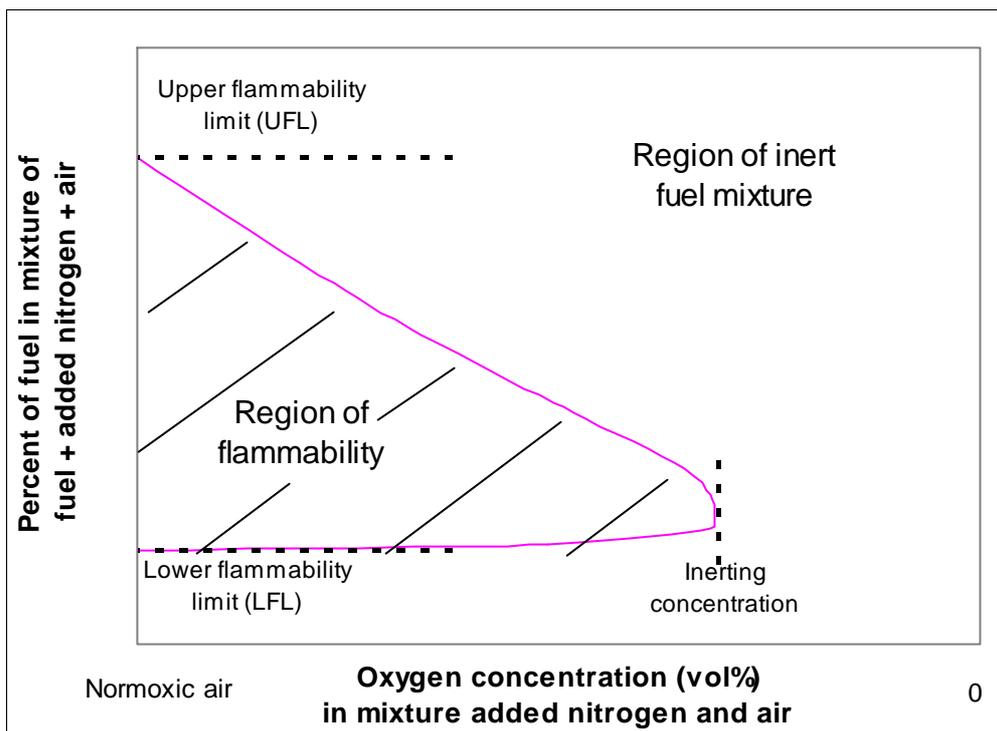
Figure F.1 Definition of inerting concentration.
