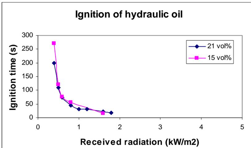
Figure H.5 Time to ignition at different radiation levels and oxygen concentrations.
