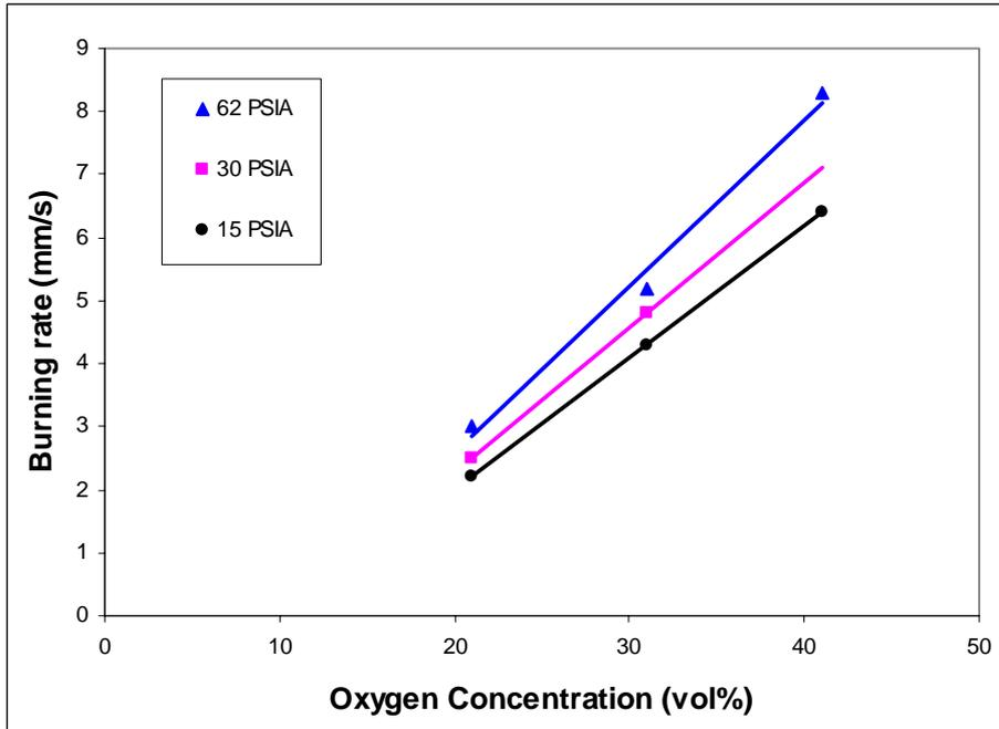
Figure 4.3 Experiments show the dependence of oxygen concentration and the small dependence of oxygen pressure on burning rate of class A material [8].
