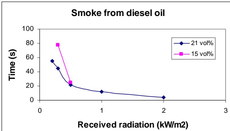
Figure 4.17 Time to emit smoke from diesel at different radiation levels and oxygen concentrations.
