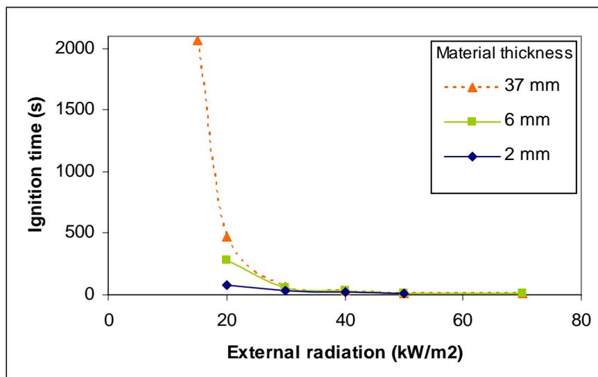
Figure 4.11 Ignition time in normoxic air for different thicknesses of spruce panels plotted as a function of external radiation [16].
