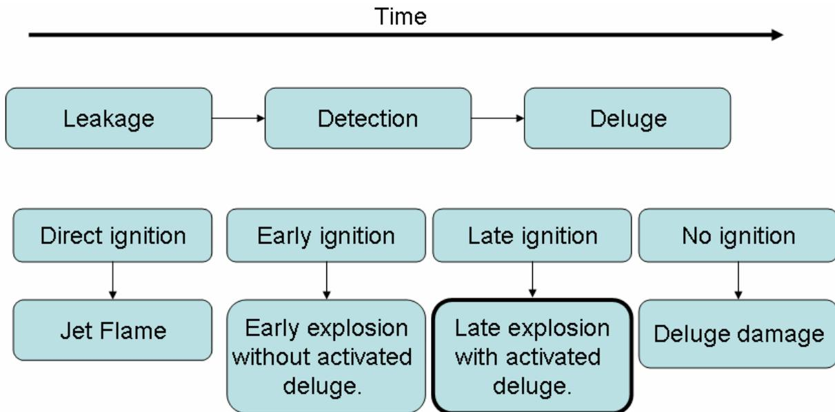
Figure 37: Illustration of the competing of time between the activation of deluge and different possible outcomes of a gas release.
