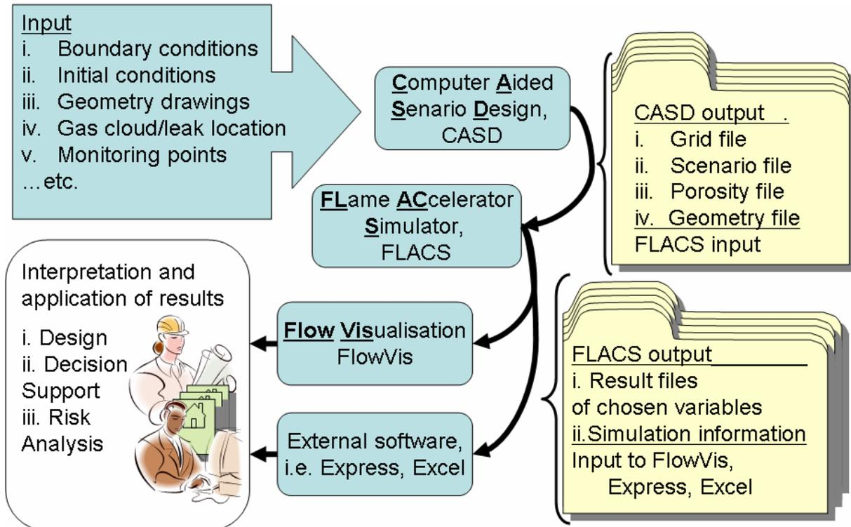
**Figure 30: Illustration of explosion modelling process with the CFD code FLACS from the start in input to the goal of interpretation and application of results.**
