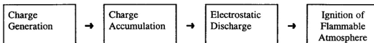
**Figure 20: A simple model of static spark ignition. From HSE (1995) “Electrostatic hazards associated with water deluge and explosion systems offshore”**
