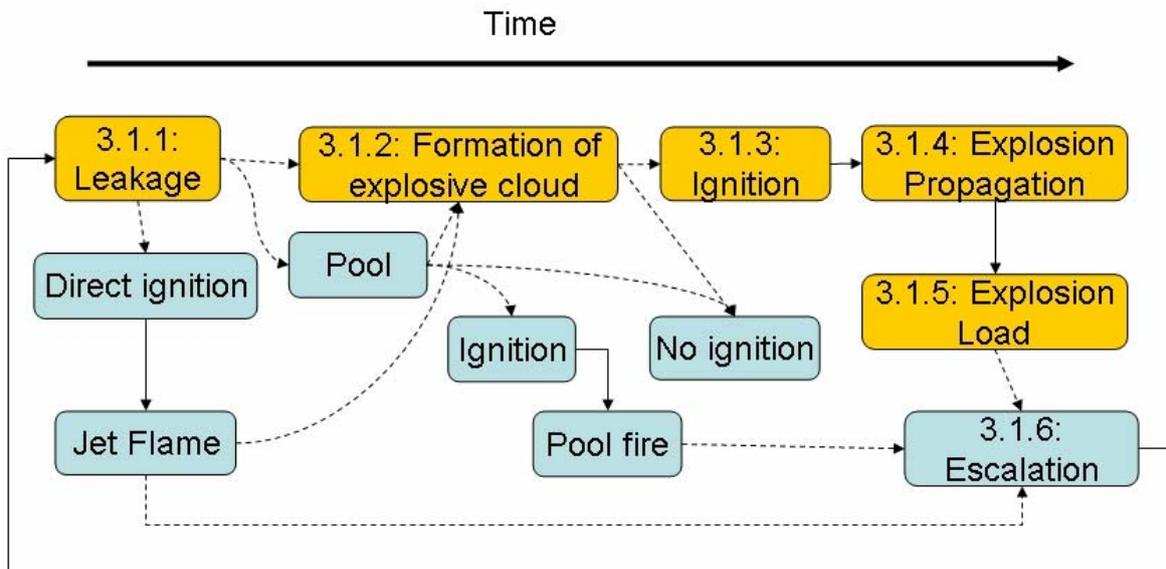
**Figure 15: A simple model for premixed gas explosions. The explosion path is emphasised by the yellow colour. Note that the model shows the chronological order of events. Dotted arrows show different alternatives on how the chain of events might develop. The explosion events have been coloured yellow. The numbers represents the chapters of this section as a logical disposition.**
