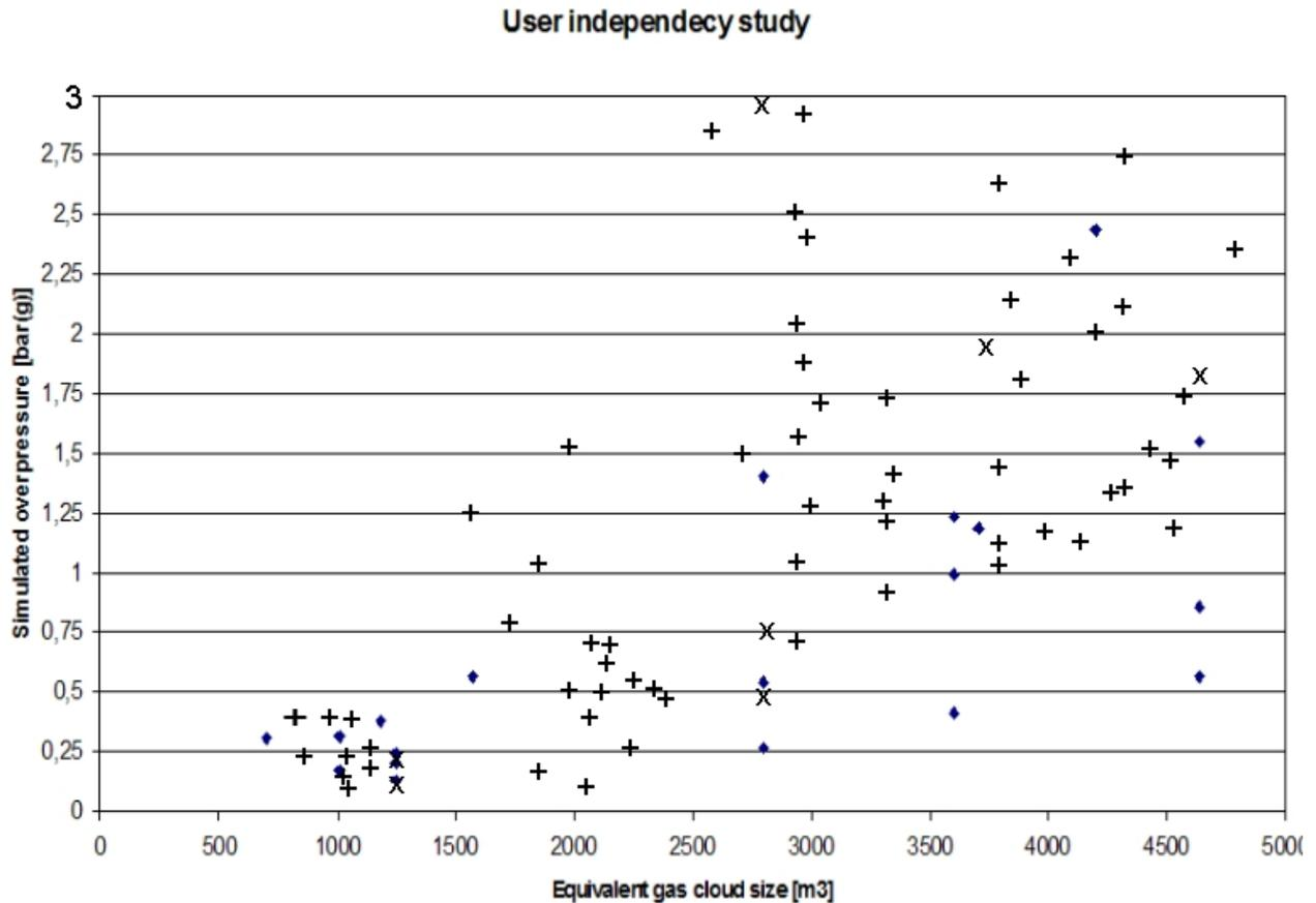
**Figure 56:** The diagram shows the results from two independent users. Results from the earlier study with a grid of 1meter was used are represented by (+). Diamonds represent simulation results from the present study using the finer 0,5meter grid, while (X) represent identical simulations using a 1meter.
