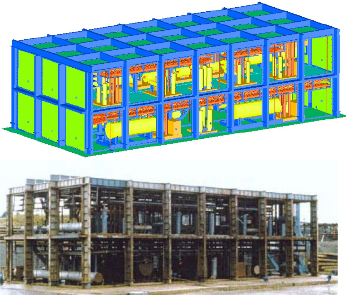
**Figure 32: A comparison of the BFETS phase 3a experiment geometry with the FLACS geometry used for validation. From Wingerden et. al. (1998) “Effect of deluge on explosion: FLACS simulations compared to full scale experiments” and HSE (2000) “Explosions in Full Scale Offshore Module Geometries Main Report” OTO 1999 043**
