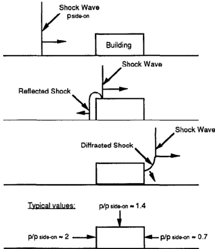
Figure 26: Illustration of reflection and diffraction phenomena when a blast wave interacts with an object. From Bjerkvendt et. al. (1997) “Gas explosion handbook”
