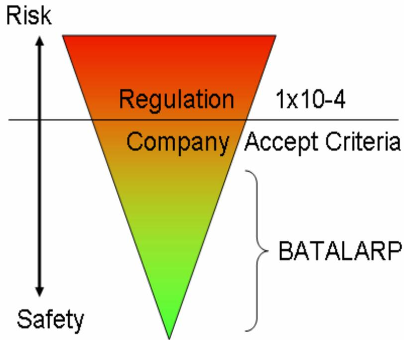
**Figure 12: An illustration of a hybrid criterion in accordance with the Norwegian offshore legislation.**
