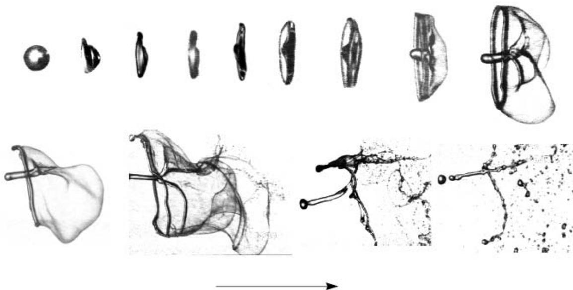
**Figure 29: High-velocity video recording of a droplet break-up. From Wingerden (2000)**
