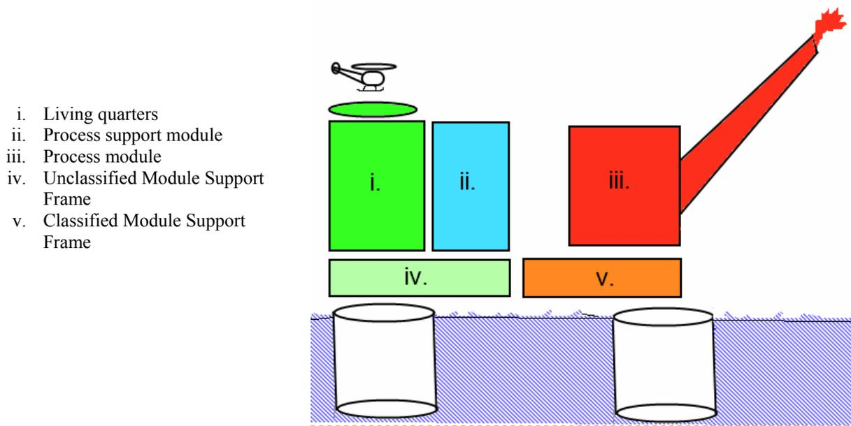
**Figure 42: Schematic illustration of the Troll B platform. The platform is constructed to separate the living quarters, helipad and process support module as far as possible from the more dangerous process module, the flare system, the risers and export pipelines.**
