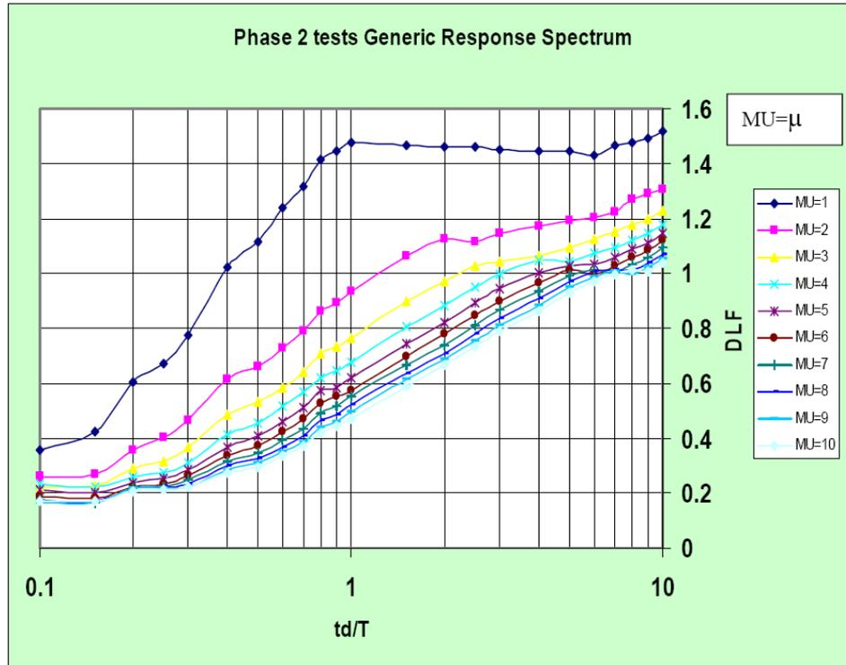
**Figure 25: Generic response spectrum diagram, from which the Dynamic Load Factor can be estimated. From HSE (2006) “Response spectra for explosion resistant design and assessment”**
