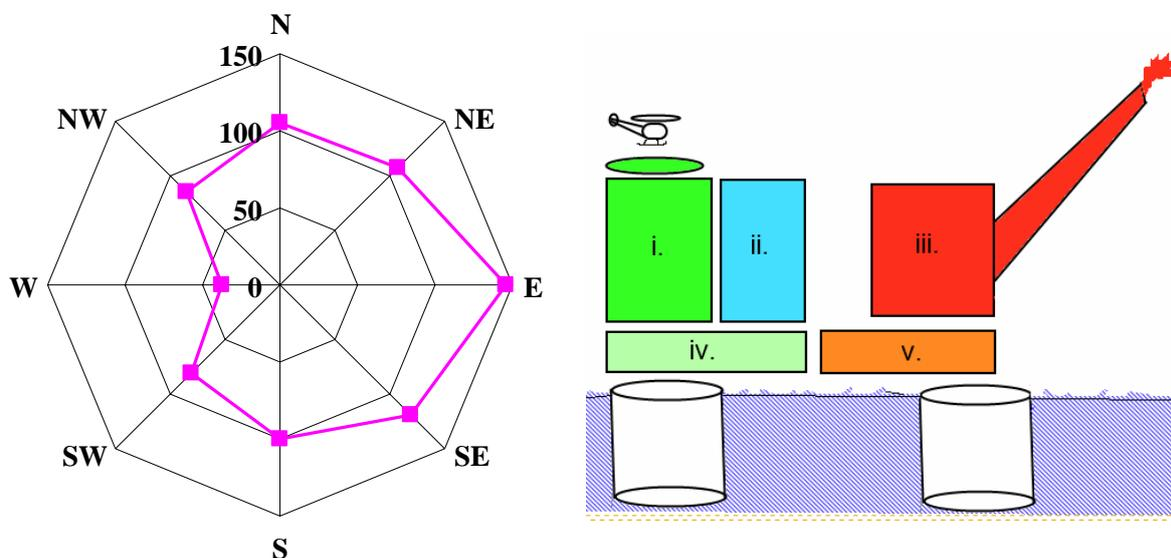
**Figure 45: Illustration of the ventilation results (left) together with an overview of the platform (right). Note that the relation between the ventilation results and the position of the process module (iii).**
