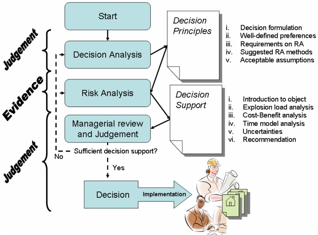
**Figure 40: A schematic description of the suggested decision framework. Note that the outputs from the Decision Analysis and Risk Analysis are represented as the Decision Principles and Decision Support documents. Based on the decision and risk management process described by Aven et. al.**
