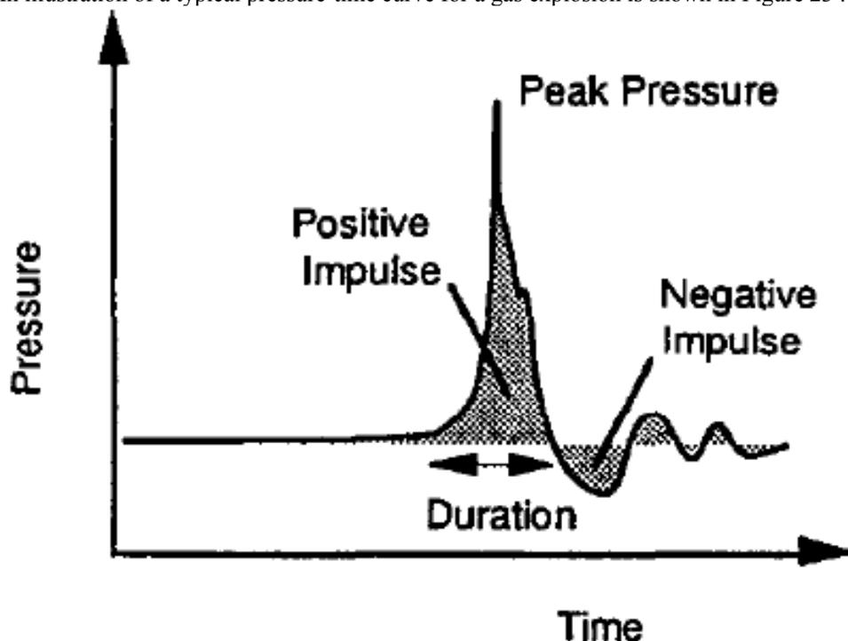
**Figure 23: Schematic description of a typical pressure-time curve for a gas explosion. Note that the definitions are explained in the picture. Bjerkvendt et. al. (1997) “Gas explosion handbook”**
