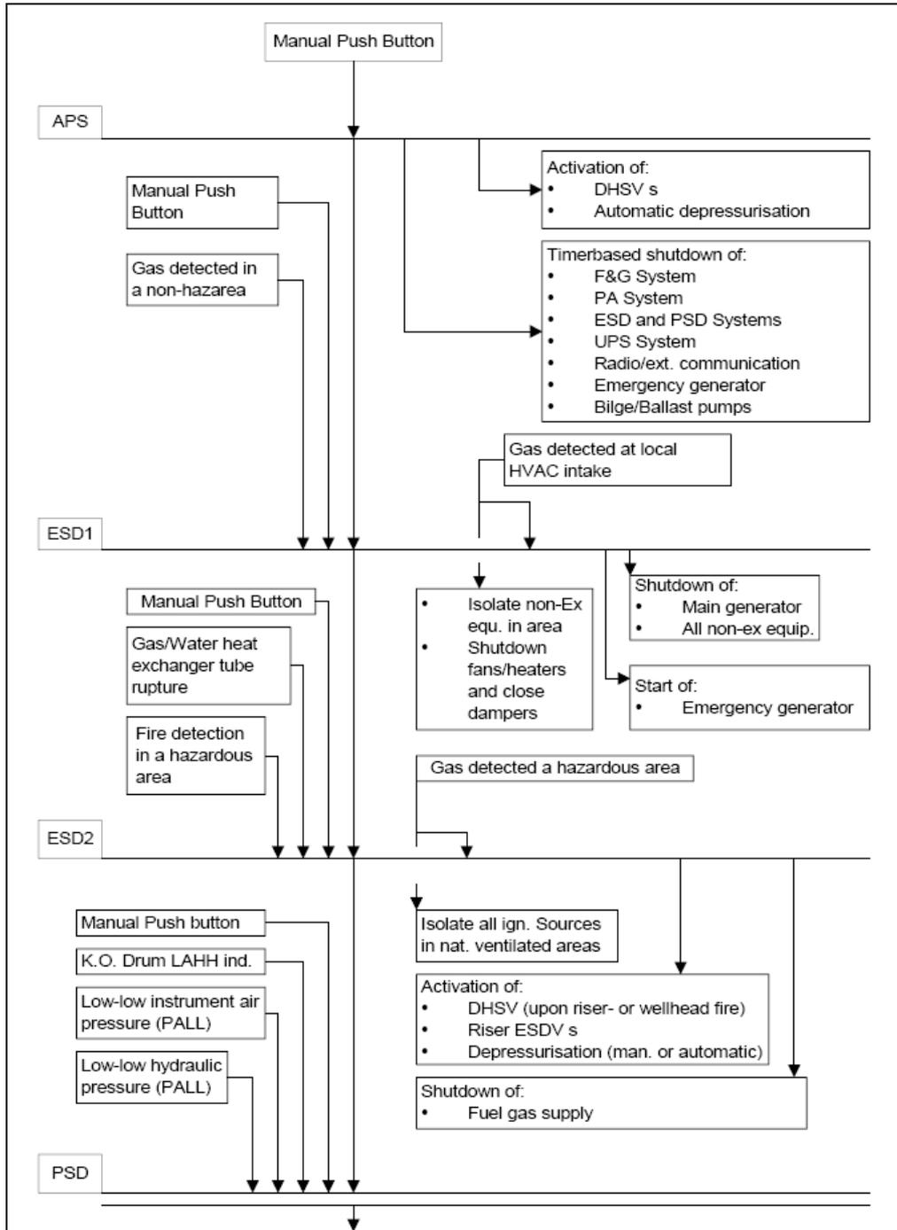
Figure 38: A simplified example of ESD hierarchy, from NOROK S-001. Activation of the higher levels automatically all the levels below. The means of activation of the different levels are also indicated by the arrows. It must be noted that the ESD hierarchy diagram used in reality are much more detailed and cover a broader set of responses.
