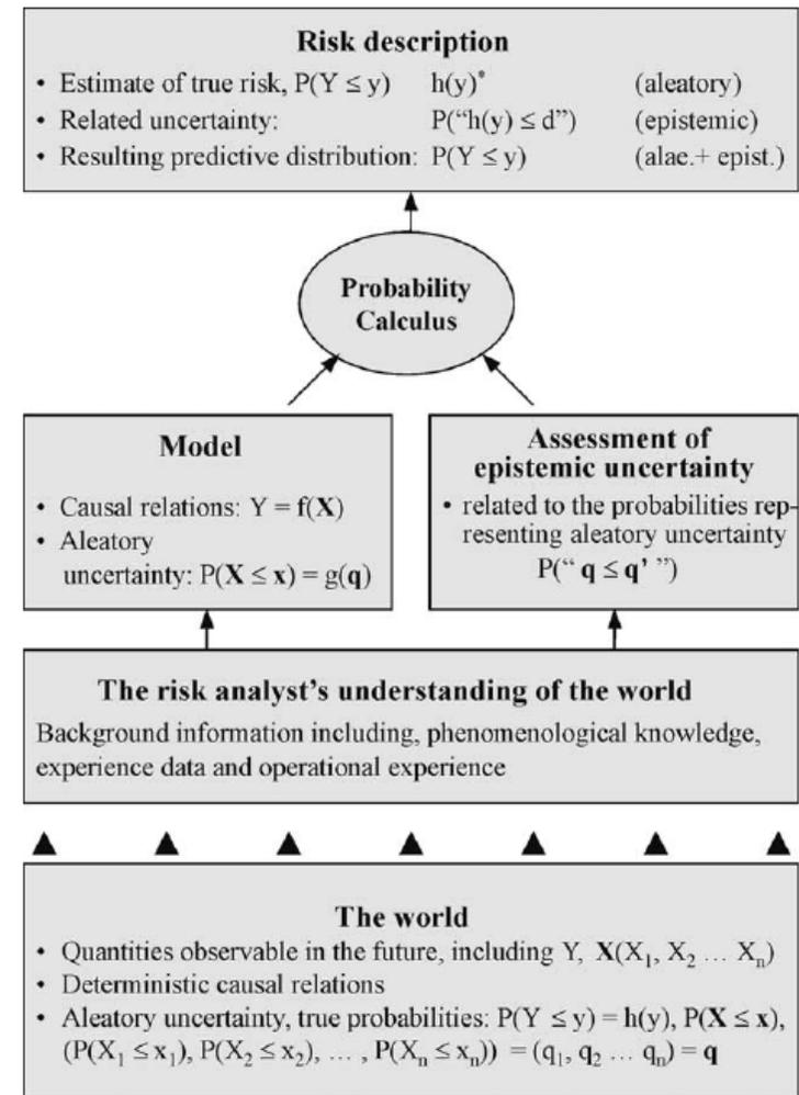
Figure 4: Comparison between the handling of uncertainties in the predictive Bayesian framework (left) and the classical risk framework (right) as presented by Nielsen et. al. The letters  $d$  and  $h$  in the right figure represent dummy variables.  $P(X)$  represent the probability of an event or quantity, while  $f(X)$  represent a model function to calculate the desired estimate quantity Y.
