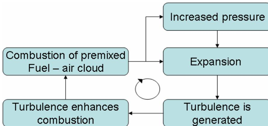
**Figure 22: An illustration of the Schelkin mechanism. From “Gas Explosion Handbook”**
