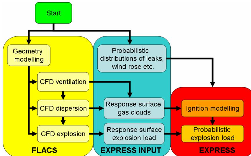
Figure 35: A Schematic description of the connections between FLACS and EXPRESS.
