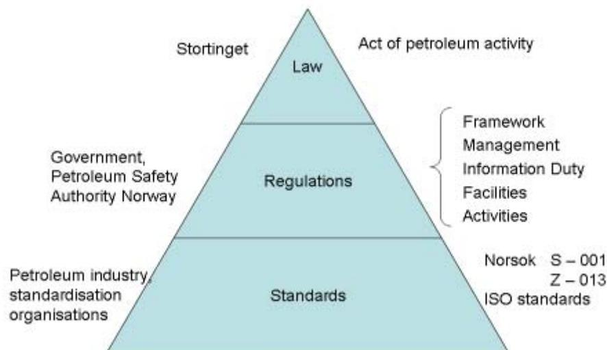
**Figure 13: Schematic description of the system of laws, regulations and standards in Norway.**
