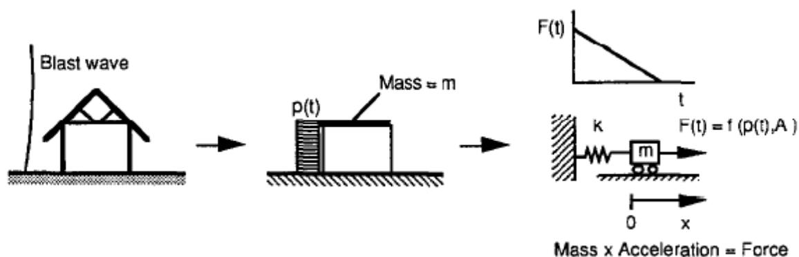
**Figure 24: An example of how a house can be reduced to a single-degree-of-freedom system**
