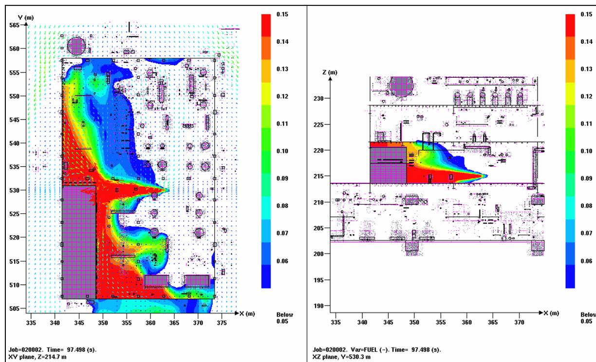
Figure 48: An illustration of gas dispersion simulation 020102. To the left a XY cut-plane of the concentration profile is shown, looking at the module from above. To the right, the same simulation is presented by a XZ cut-plane showing the concentration profile from the side, looking in the Y-direction. The arrows in the left picture illustrates the wind vectors.
