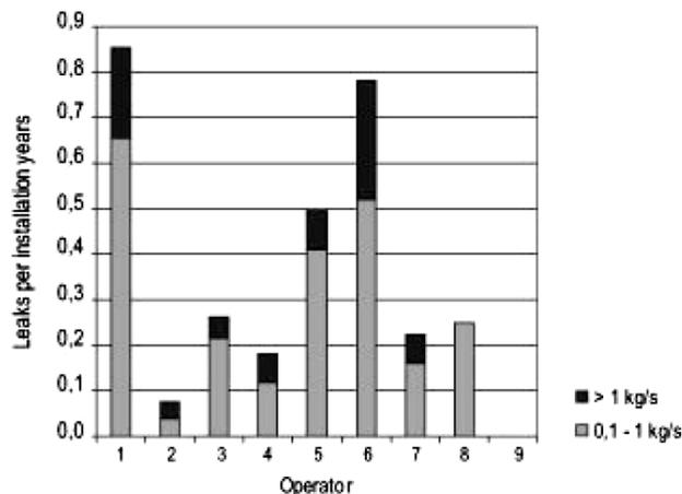
**Figure 17: Diagram over the average leak frequency per installation year for nine anonymous operating companies on the Norwegian shelf<sup>96</sup>**
