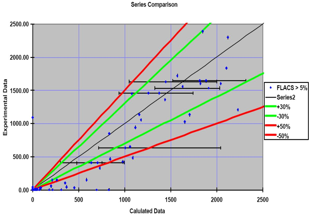
**Figure 34: Comparison between gas dispersion predictions using FLACS and full-scale experiments. The diagram shows gas cloud volume with a concentration above 5%, which is typically the lower flammability limit of natural gas. From Savvides C. et. al. (2001) "DISPERSION OF FUEL IN OFFSHORE MODULES: Comparison of Prediction Using FLACS and Full Scale Experiments", available at [www.gexcon.com](http://www.gexcon.com)**
