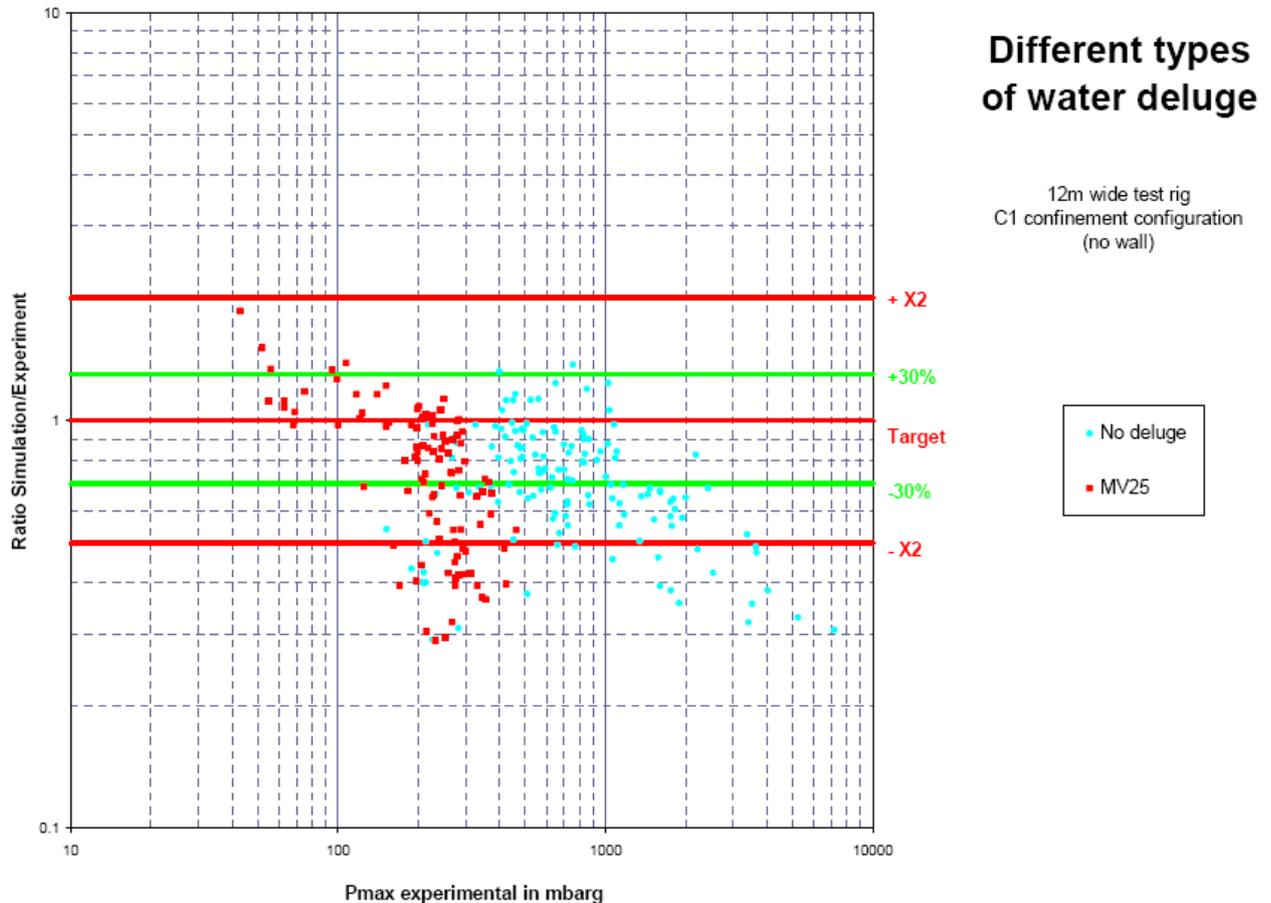
**Figure 33: Comparison between experimental data and FLACS simulations for explosions with and without deluge. Although the scales are a bit confusing, the diagram shows that the majority of predictions are approximately within a factor between 0,5-2.**
