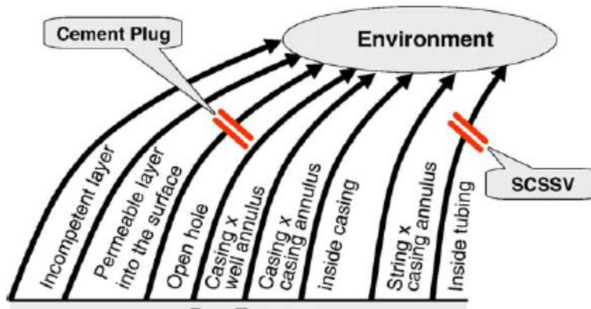
**Figure 19: Totality of possible fluid flow paths between well and the environment, with two examples of well safety barriers. From Miura et al.<sup>100</sup>**
