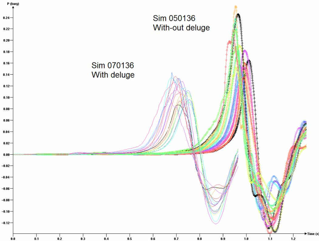
**Figure 52: The pressure-time history at the measuring points for two simulations only different in the use of deluge in 070136 and no deluge in 050136. Note that the pressure is reduced from 0,25 bar(g) to approximately 0,14 bar(g) in this particular example.**
