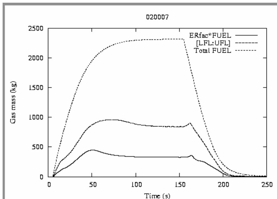
**Figure 46: Example of dispersion simulation 020107 with a large mass flux (100 kg/s) combined with a wind speed of 8.5 m/s with opposite direction to the leak .**
