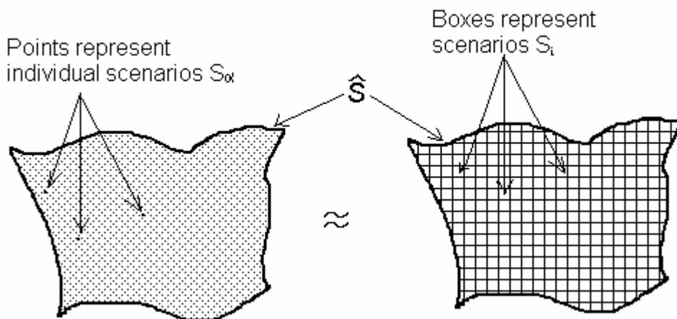
**Figure 2: The figure illustrates a geometric representation of the quantitative risk definition used by Kaplan. To the left is a representation of the infinite set of risk scenarios which defines  $R$ . To the right is the partitioned, disjoint set representing  $R_p$ . From Kaplan S. et. al. (2001) “Fitting Hierarchical Holographic Modeling into the Theory of Scenario Structuring and Result Refinement to the Quantitative Definition of Risk”**
