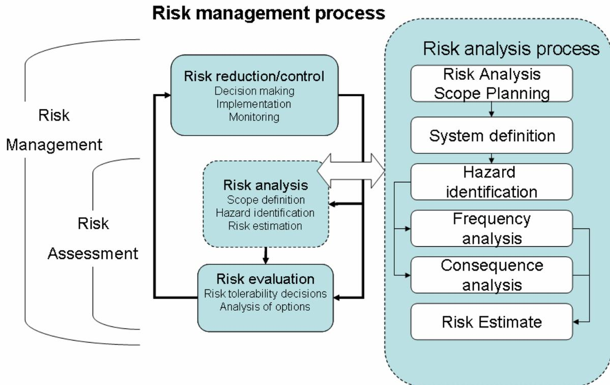
**Figure 6: Schematic illustration of the relations between risk management, risk assessment, risk evaluation, risk analysis and decision making in the risk management process. Based on IEC (1995) "International standard 60300-3-9, Dependability Management – Part 3: Application Guide – Selection 9; Risk analysis of technological systems",**
