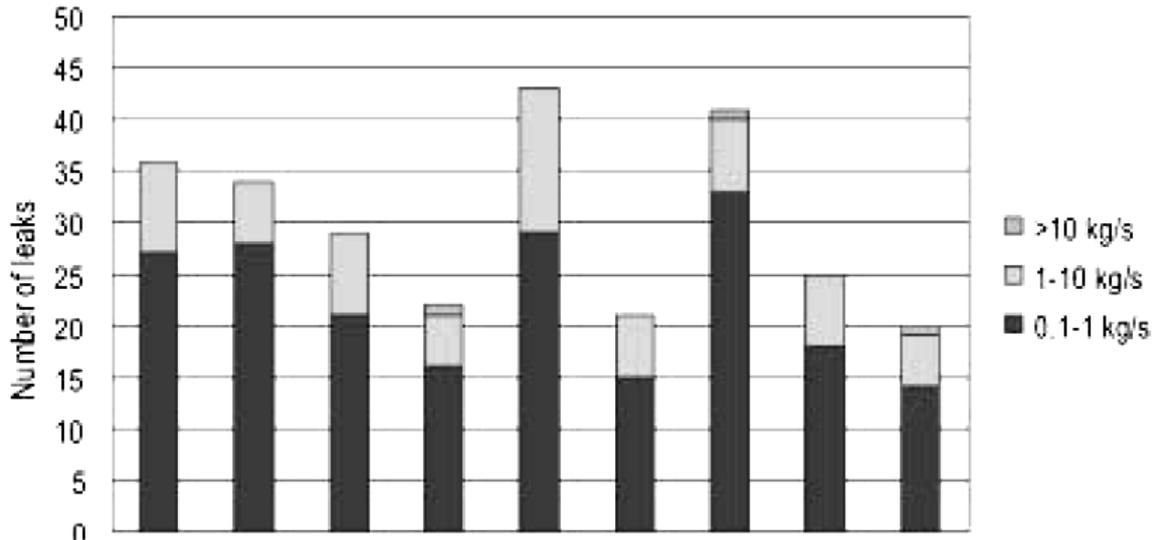
**Figure 16: Diagram showing the numbers of leakages during 1996 – 2004 on the Norwegian shelf, distributed over three mass flux classes.**
