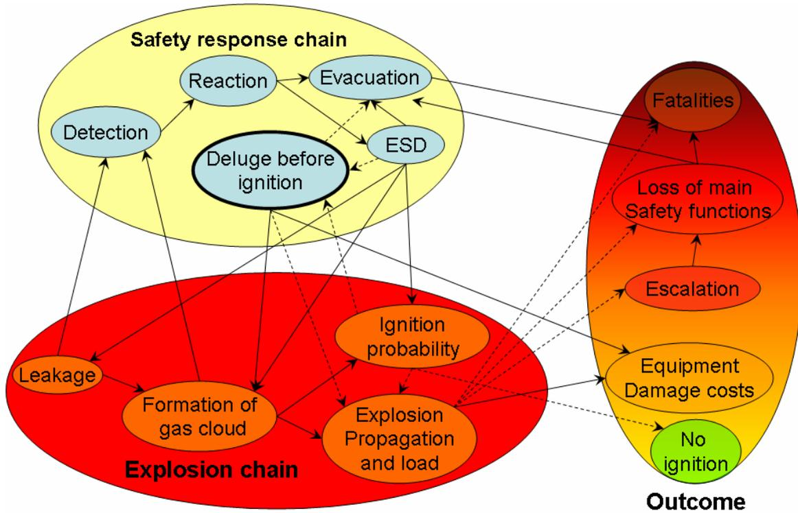
**Figure 39: Influence diagram to show the complexity of the decision whether to implement deluge as an explosion mitigation measure or not. Thick arrows indicate a certain influence, while dotted arrows indicate possible influence, depending on the circumstances.**
