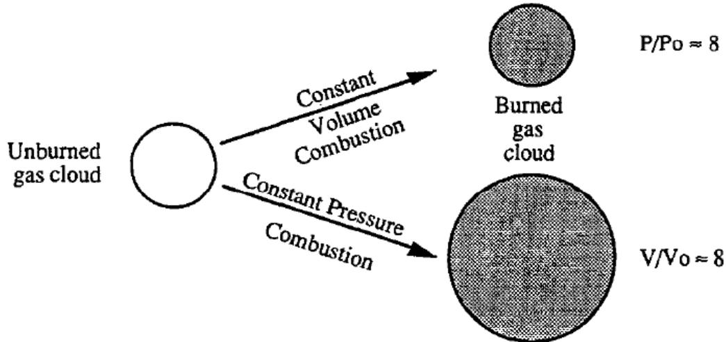
**Figure 21: Constant volume and constant pressure combustion respectively. From Bjerkevendt et al (1997) “Gas explosion handbook”**
