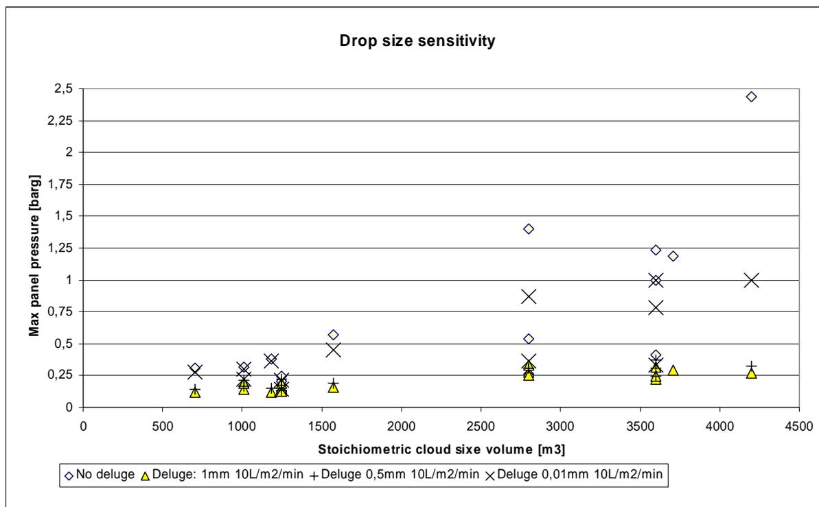
**Figure 53: The results from the drop size sensitivity study. The Maximum recorded panel pressure in each simulation has been plotted against the stoichiometric cloud size volume.**
