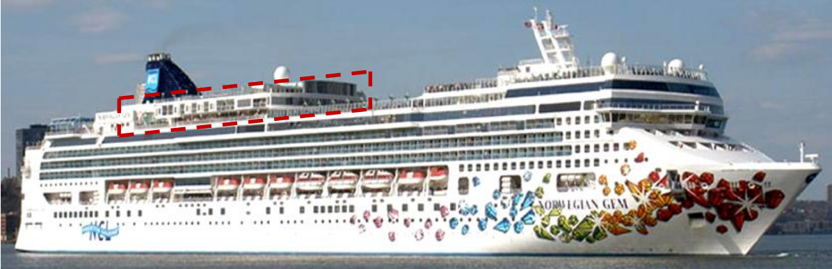
Figure C1. The Norwegian Gem and the intended FRD superstructure marked in the mid-aft section.
