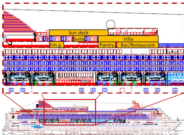
Figure 7.4. Illustration of the six locations for the design fire scenarios. (Plan: Meyer Werft)
