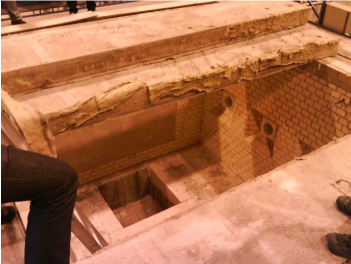
Figure 4.1. Furnace for testing deck specimens in the standard fire test.
