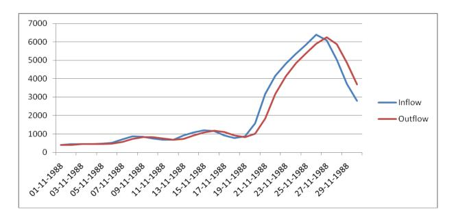
Figure 4-3 The result of flood wave routing in the Pahang River reach from Lubuk-Paku gauging station to the junction River Gelugor of the main river.
