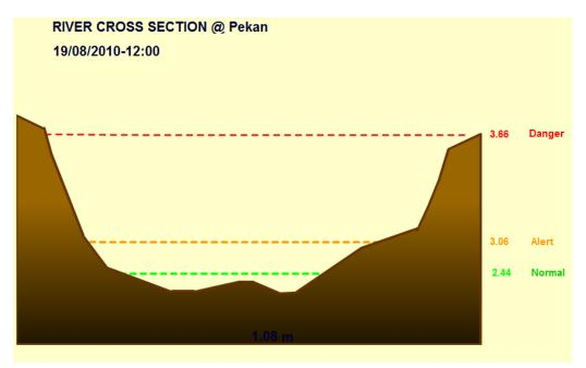
Figure 5-4 the normal, alert, and dangerous water level of the river Pahang at Pekan(malaysian Meteorological Department).
