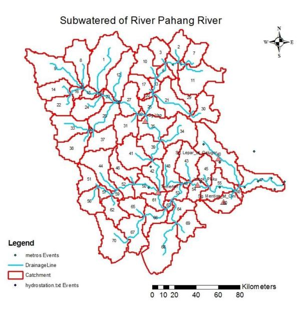
Figure 2-1 Sub-watershed delineation and polygon processing, each polygon represents the sub-watershed in the basin with the respective numbers. The area of the polygons can be seen in Appendix A. The total area of the entire basin is estimated to be 27000km<sup>2</sup>.
