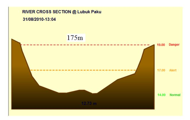
Figure 3-6 The cross section on the river at Lubuk-Paku gauging station (Malaysian Meteorological Department station Id,3527410)
