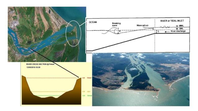
Figure 5-2 Definition sketch of the wave setup at a river mouth and river cross section (Google earth, Hitoshi, T., and Nguyen, X. T., 2008)
