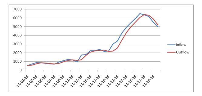
Figure 4-4 The result of flood wave routing in the Pahang River reach from the junction of River Gelugor to Pekan. The distance between thus two points is 71km.
