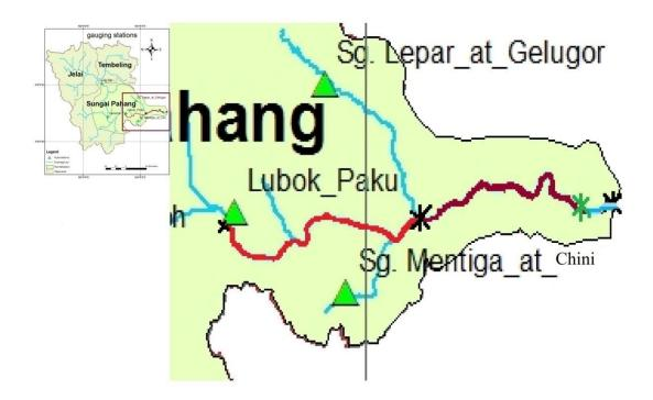
Figure 4-2 The river reach where the two step routing processes have taken place. The red line indicates the first step routing and brown line shows the second step routing
