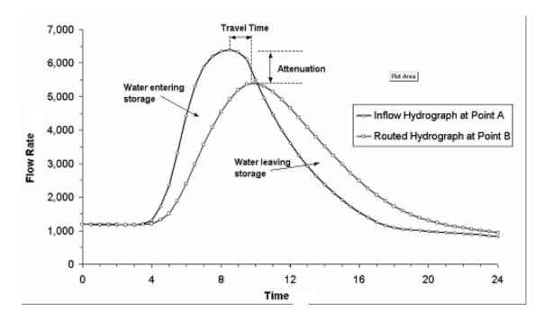
Figure 4-1 Translation and storage processes in stream channel routing (Ponce, 1983)
