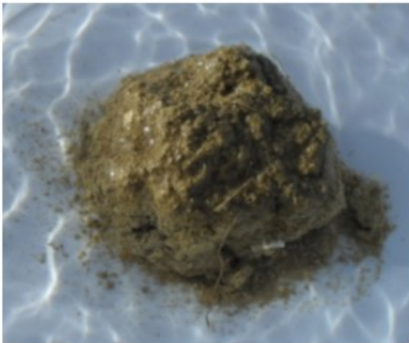
Figure 20; Soil aggregate test to study the durability of a soaked sample.
