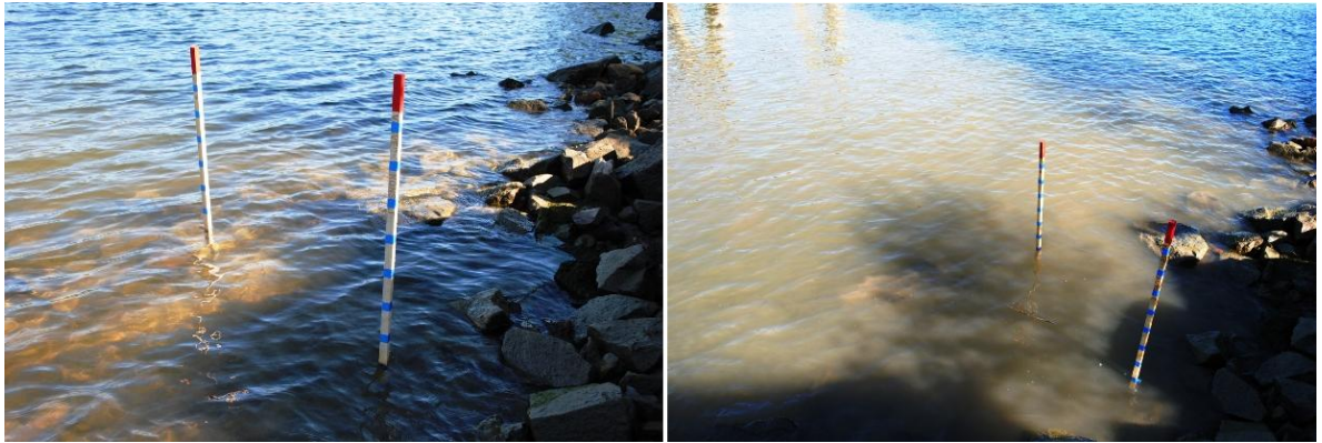
Figure 21 - Poles secured in the bottom at Garn station. The blue markers are evenly spaced 10 cm apart. The left picture was taken just before the passage of the ship Patria. The right picture was taken about five minutes after the ship had passed Garn station. Notice the large increase in turbidity (© Althage 2010).
