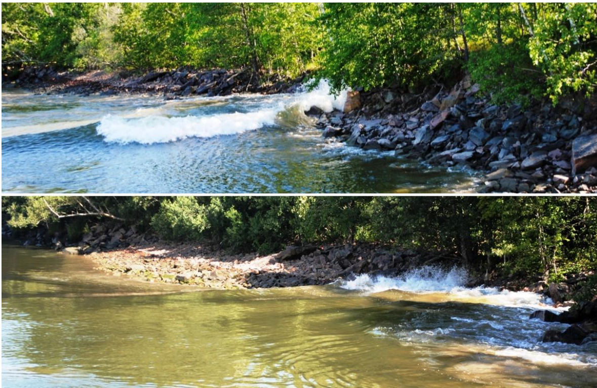
Figure 17 – Wave troughs following the drawdown after two ship passages. The top picture is taken on 2010-06-04 when the ship Patria was navigating the river. The bottom picture is from 2010-08-02 during a passage by Birthe Bres. Note how high up on the bank the waves break, reaching as far as the vegetation line (© Althage 2010).
