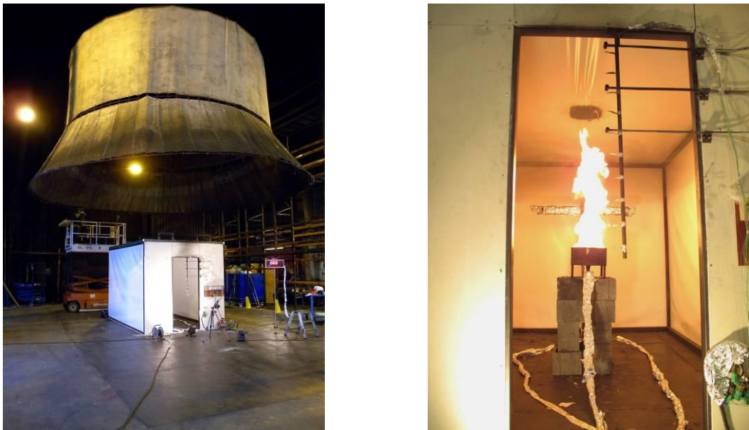
Figure 5. The test set-up for the large-scale tests with textile membranes conforming to the size of the ISO 9705 room, 2.4 m × 2.4 m × 3.6 m (left), and the position of the burner in the centre of the room in one of the validation experiments (right). (1)
