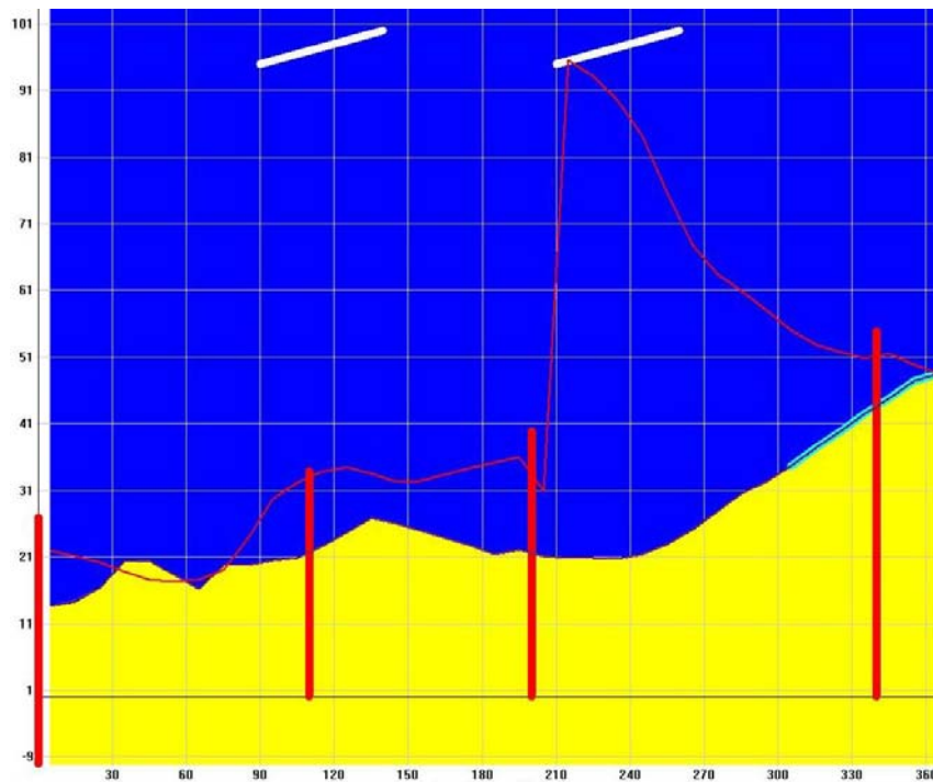
Figure 12.3 Detached breakwater performance, scenario H1 in 2030
