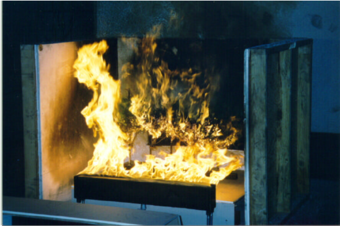
Figure 6.10: 30 seconds after ignition, approximately 250 kW.
