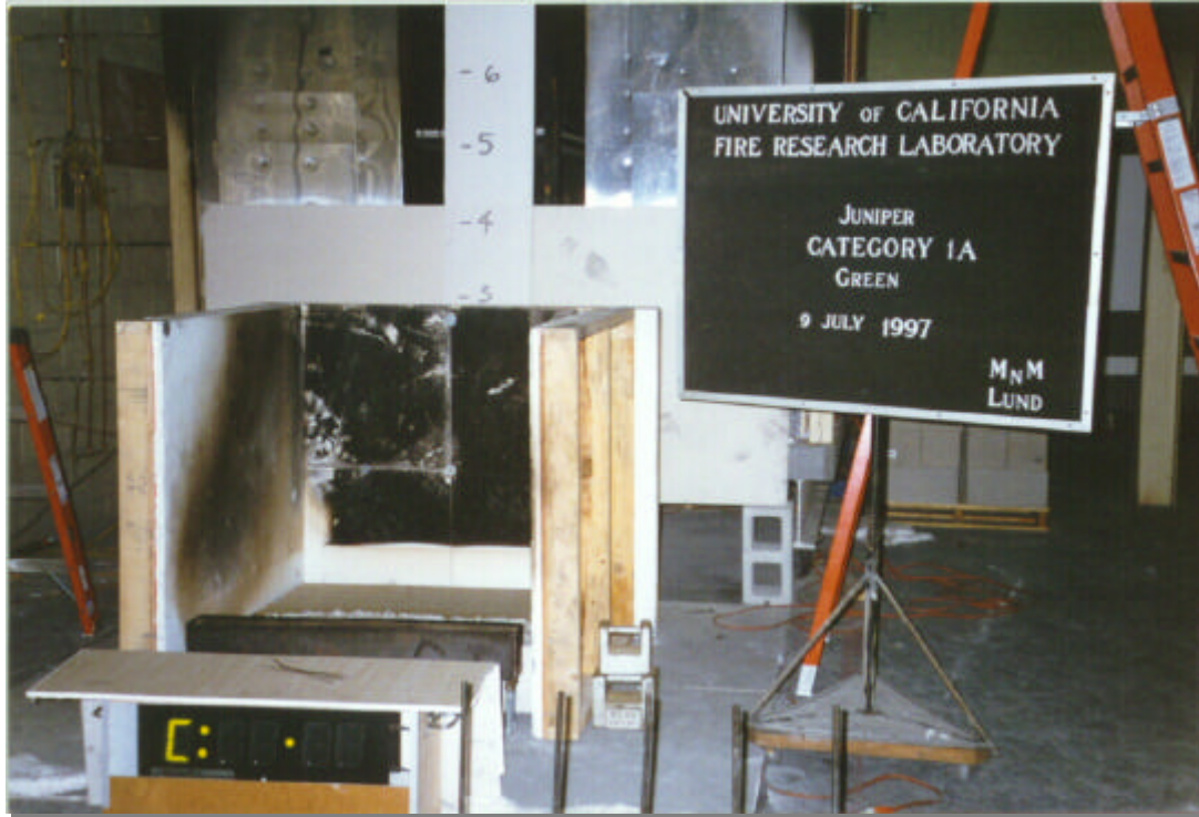
Figure 6.4: The burning setup seen from the front.
