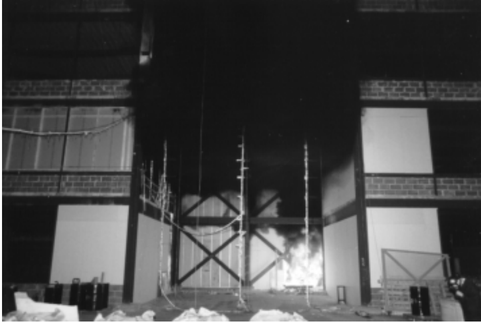
Figure 3.3 Photo from one of the experiment showing the external opening. Photo by S-I. Granemark
