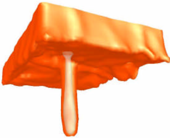
Figure 3.2, Smoke filling with the 2.7 MW fire
