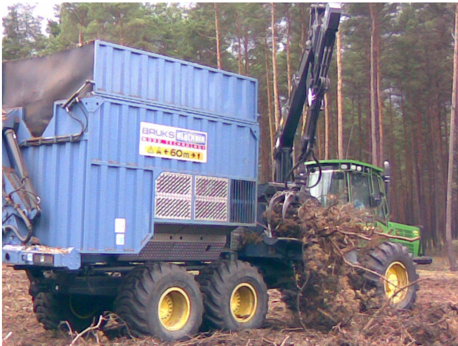
Figure 6-4 Modern mobile Bruks chipper equipped with container
