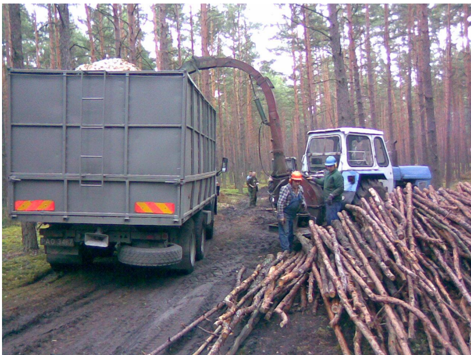
Figure 6-5 Manually fed chipper
