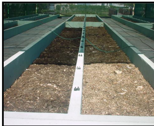
Figure 2-5 Concrete vermicomposting beds.
