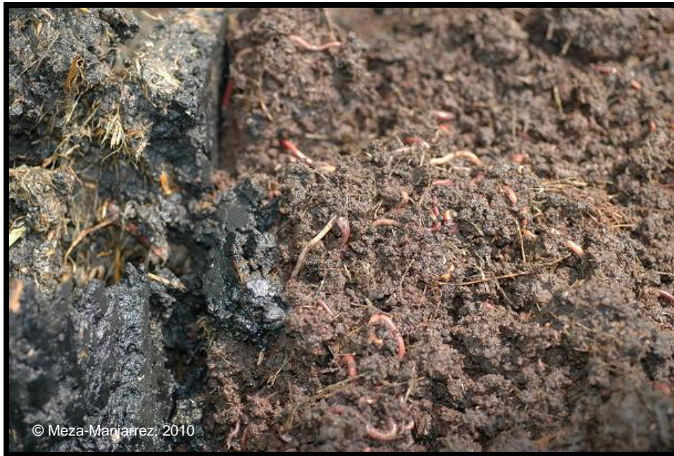
Figure 2-3 Decomposition of sewage sludge by earthworms. Unprocessed sludge (left-hand side) results from the lack of porosity due to insufficient bedding material.
