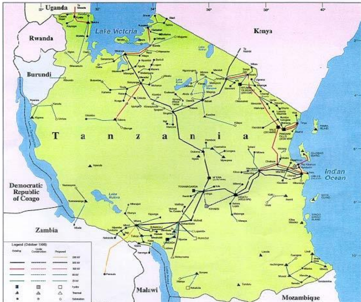
Figure 5-1: Map displaying the extent of the electricity grid in Tanzania in 2009. Source: (Kabaka & Gwang'ombe, 2007)
