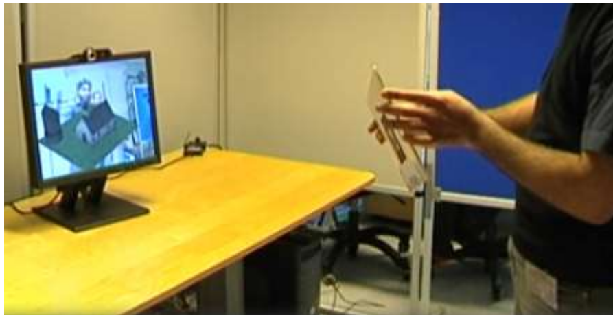
Figure 5-12 A user having Active Interaction by holding the marker (model) while the manipulated model is shown in the display pasted over top of it.
