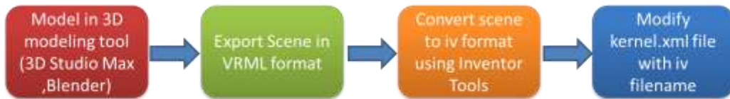
Figure 5-9 Steps required to port 3D scene from a modeling tool to a Studierstube based application
