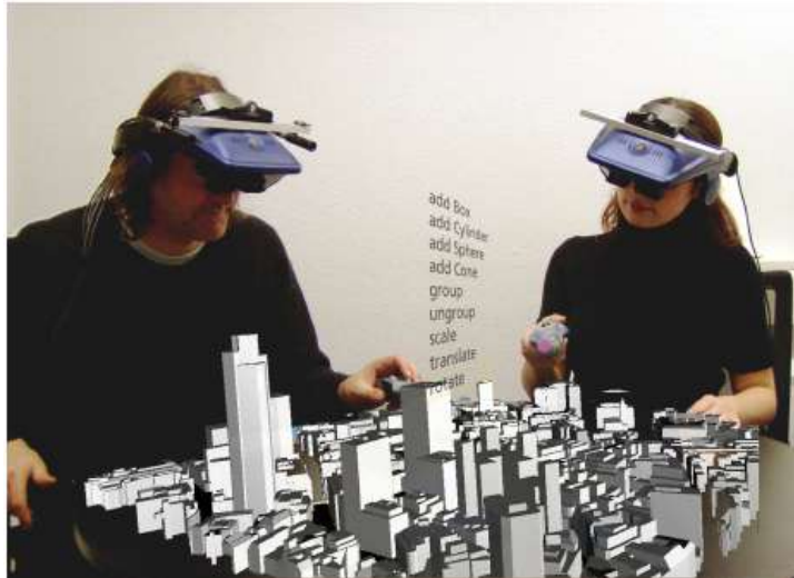
Figure 3-3 Architects using see-through HMD for collaborative Augmented Reality urban planning in the Arthur Project [22]
