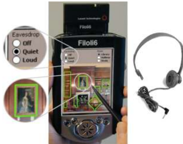
Figure 2-5 Figure illustrating Electronic Guidebook which uses groupware software to provide user with cooperation based shared interactive experience [10]
