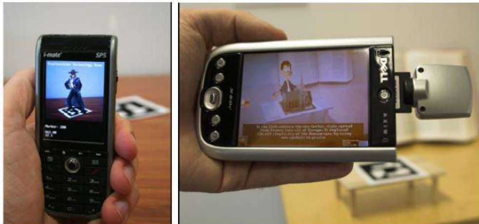
Figure 3-7 (Left) A marker-based AR application on a commercial cell phone showing a 3D character pasted in reality (Right) A marker-based AR on PDA showing a 3D character explaining information about a church model in front of him [23]
