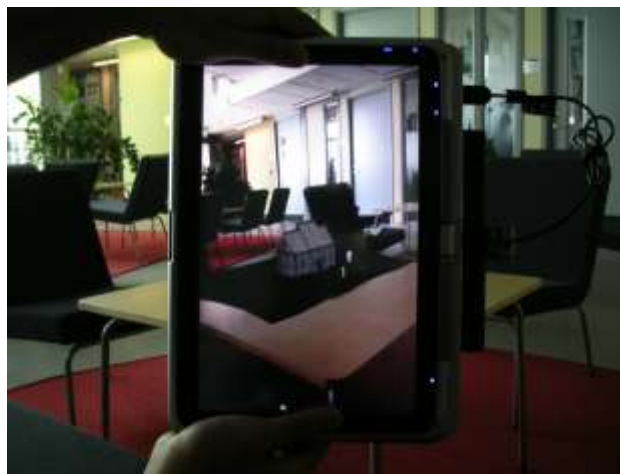
Figure 5-25 A user holding the device vertically to experience the table top augmented model
