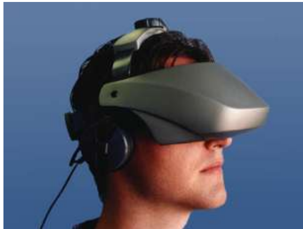
Figure 2-1 A user wearing HMD for interactive Virtual Reality experience with 3D Virtual Scene (Image courtesy: www.5DT.com )
