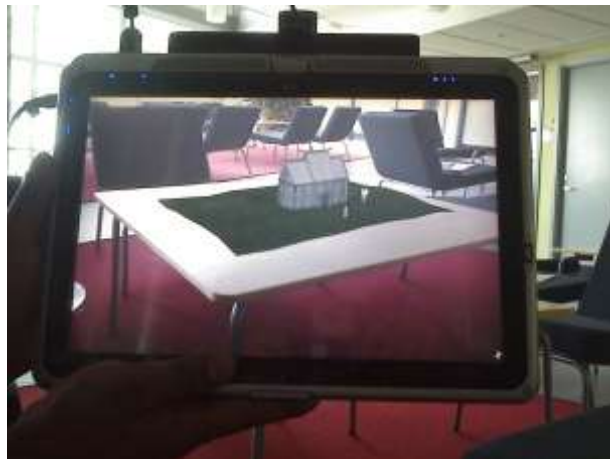
Figure 5-24 A user holding the device horizontally to experience the table top augmented model
