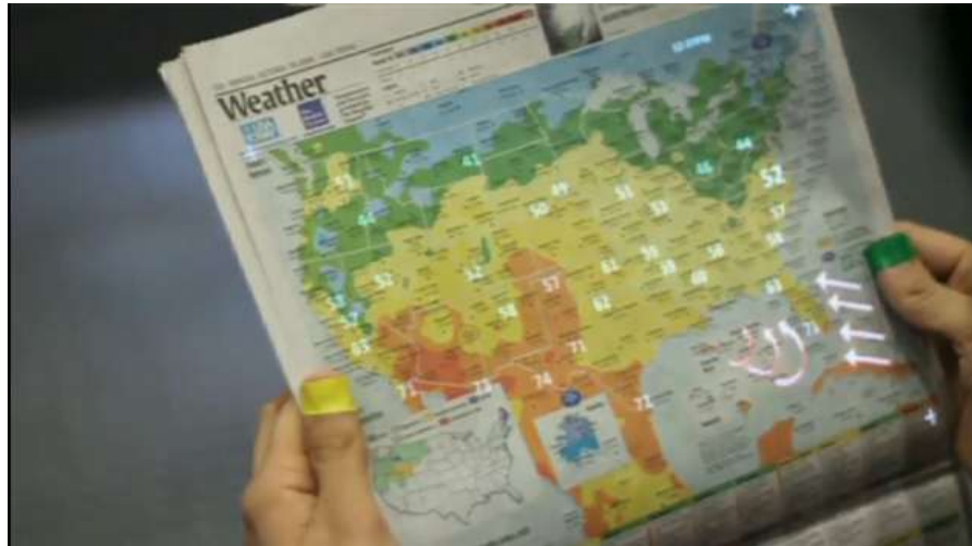
Figure 3-5 Projective Augmentation used to display interactively updated information on a weather forecast page in a newspaper (MIT Sixth Sense project)
