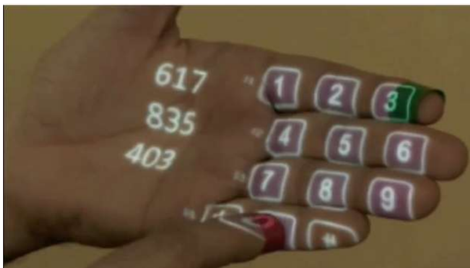
Figure 3-4 A virtual Dial pad is Projected and Augmented with the user's hand in the MIT Sixth Sense project
