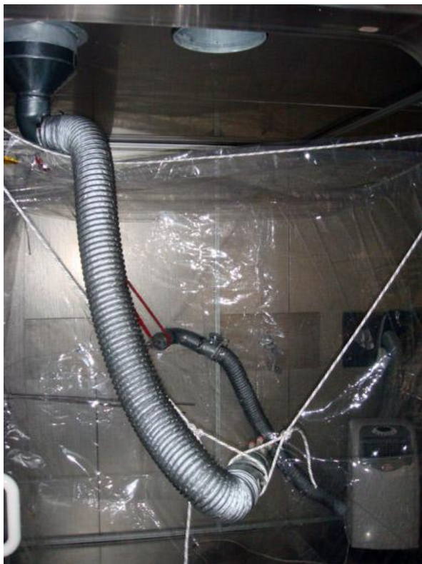
Figure 3.14: The Teflon chamber and air inlet/outlet connections.
