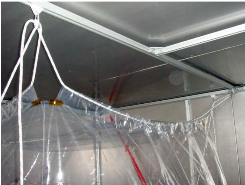
Figure 3.16: The suspending system of the Teflon chamber.
