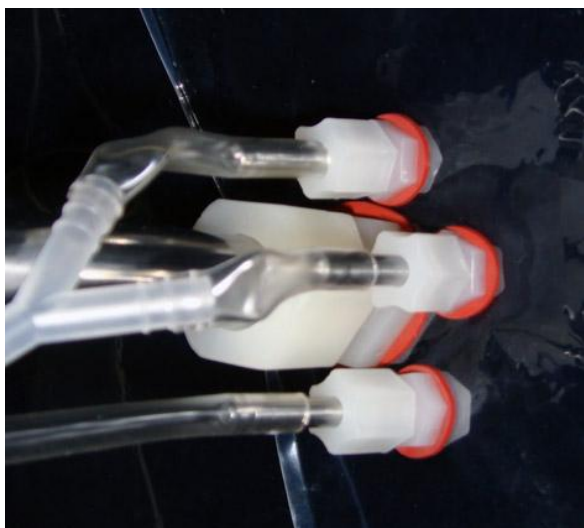
Figure 3.17: Kynar fittings on the Teflon chamber.
