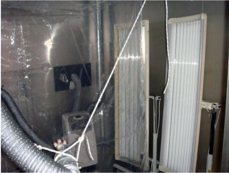
Figure 3.15: Measurement setup with Teflon chamber, AC and UV armatures.
