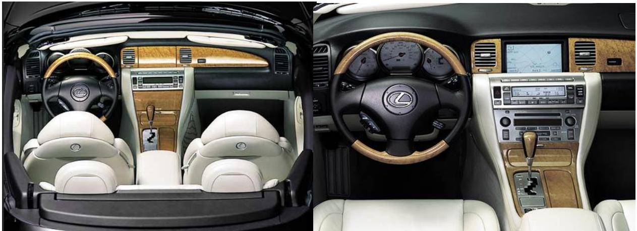
Figure 4.3: Two pictures from the same car (a Lexus) show a way to remove the first frightening impression that a huge set of buttons could create. In the picture to the left all buttons and the display are uncovered but in the picture to the right buttons for functions not in use are covered.
