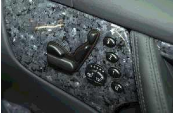
Figure 4.5: Mercedes has come up with a perfect and understandable system to adjust the seats. The buttons could relatively easy (by the user) be connected to the functions (in this case the electrical seat adjustments) that they are meant to control.
