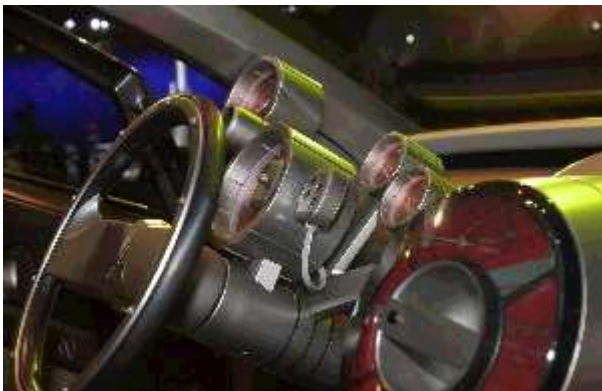
Figure 4.7: This picture shows a concept car from Mitsubishi and is a good summary of what many concept cars (cars with ideas of the future) from different companies are heading for. In this picture (in the right, lower part of the picture) the control is a huge handle. In many new cars on the market you will find many buttons and controls but in the concept cars there is one or just a few controllers and these are in many cases very big. Another example of this type of ideas in concept cars for the future is the Mercedes pictures below:
