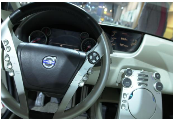
Figure 4.4: An idea to increase safety when controlling functions while driving could be to put the controls on the wheel as in this example (a Volvo concept car).
