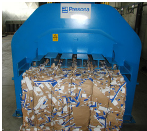
Picture 5. Machine for compressing waste
