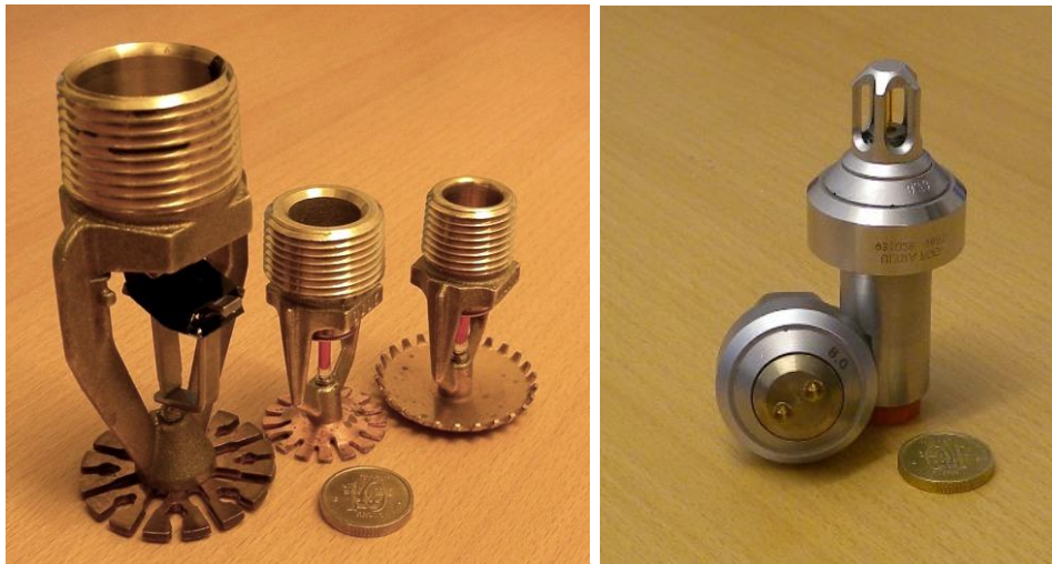
Figure 3.5 Sprinklers and water mist nozzles with different K-factors, from left: K = 17.3 , K = 11.5 , K = 8 , K = 0.08 , K = 0.073
