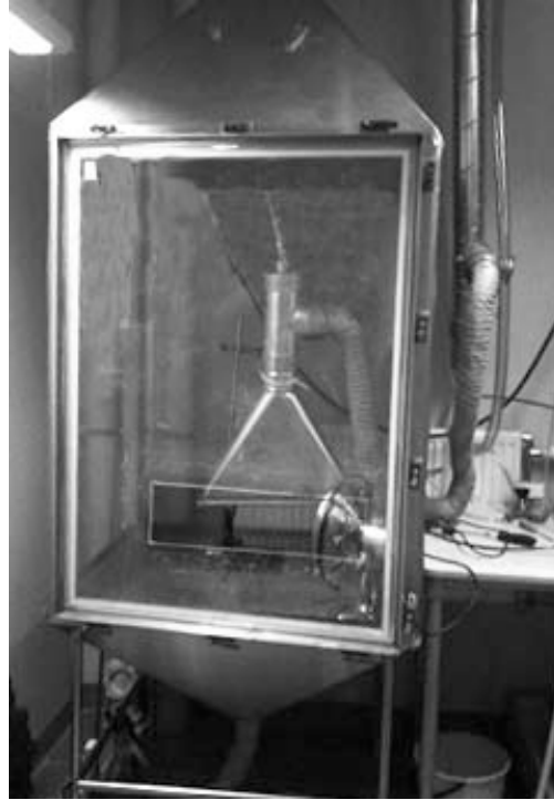
Figure 4.5. Aerosol generation system. The hole on the front is used to start a generation and is then covered with a plastic sheet to ensure no contamination of the aerosol or of the laboratory air.
