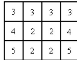
Figure 8: Example of contradicting flow directions. The numbers in the cells represent DEM elevation values. According to the equations governing flow directions, the two centre cells will be assigned opposite flow directions. To solve this water flow between the two cells are prohibited. In the single-flow model this turns the cells to sinks, whereas in the multi-flow model all the runoff is distributed between the remaining cells with elevation = 2.
