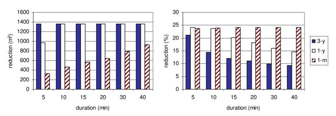
**Figure 11.** Volume reduction in thousand  $m^3$  (a) and share of total precipitation (b) for total area with the use of green roofs. Initial water levels are 50%. Design scenarios for 3-year, 1-year and 1-month rains are presented.
