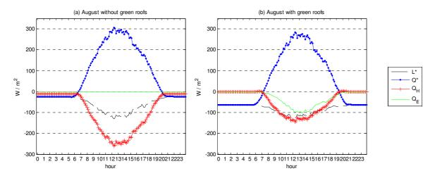
Figure 15. August simulation without (a) and with (b) green roofs.
