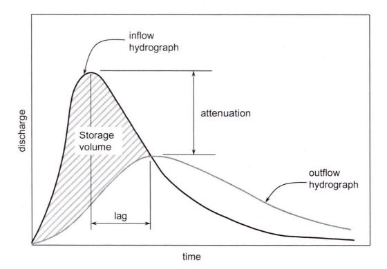
**Figure 1.** Stormwater retention (lag) and attenuation (peak reduction) with the use of BMPs. Source: Villarreal, 2004.
