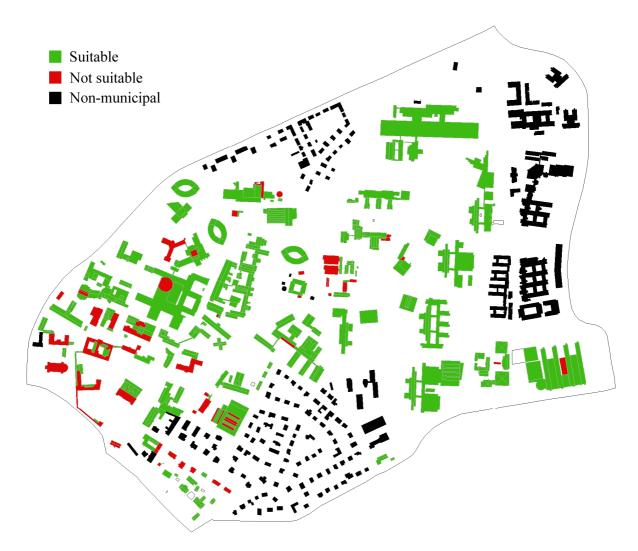
**Figure 9.** Buildings divided into roof sections. Areas suitable for green roofs are shown in green and unsuitable roofs are in red. Black buildings are non-municipal.
