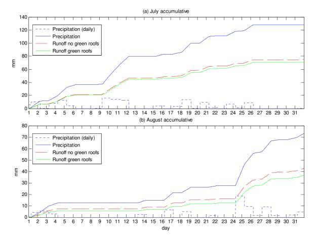
**Figure 17.** Accumulated precipitation and runoff with and without the use of green roofs for study area under July (a) and August (b). Note the different scaling on the y-axis.
