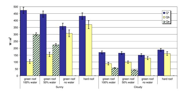
**Figure 10.** Bitumen vs. green roof comparison using a Monte Carlo simulation. Average values are shown with error bars indicating standard deviation.  $Q_H$  and  $Q_E$  are shown with positive values instead of negative.
