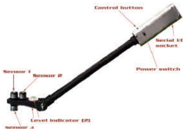
Figure 4 - TRAC instrument (Leblanc et al., 2002)
