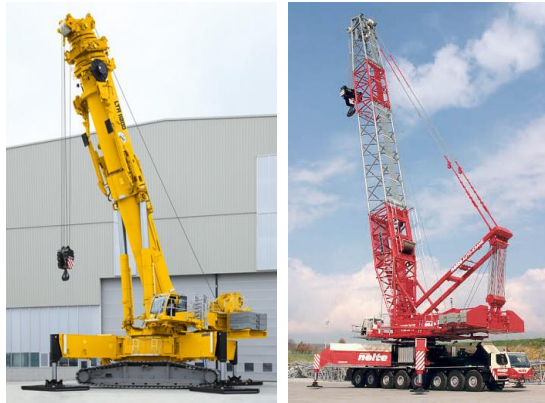
Figure 10. Crawler and truck-mounted cranes 145
