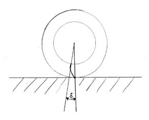
Figure 7. Sideview of tyre, showing the torsion of the carcass.
