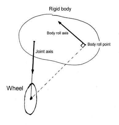
Figure 9. Model of a prismatic suspension atached to a rigid body.
