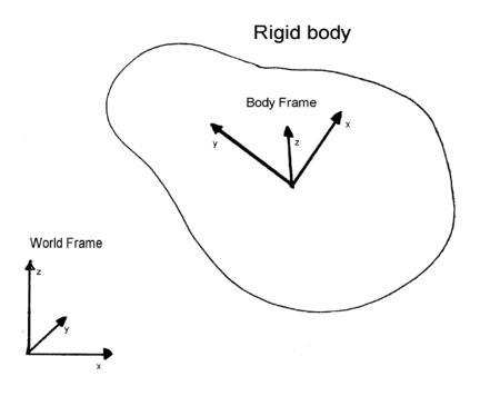
Figure 5. Rigid body with attached reference system, the body frame.
