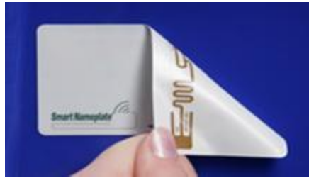
Figure 14 Example of RFID tag attached to a label ( http://www.kennedygrp.com/ , 2009-11-24)
