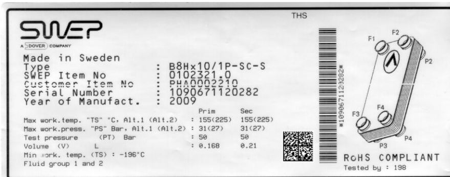
Figure 33 Silver label with Data Matrix (32*32) holding up to 91 alphanumeric characters
