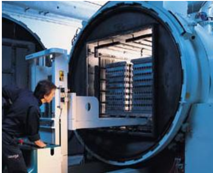
Figure 20 Pallet of BPHEs in furnace
