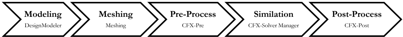
Figure 28. ANSYS Workbench simulation process.
