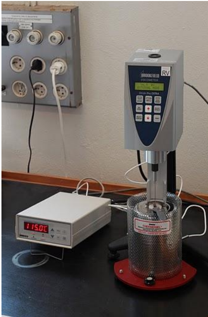
Figur 8. BROOKFIELD VISCOMETER DV-II+ Pro EXTRA
