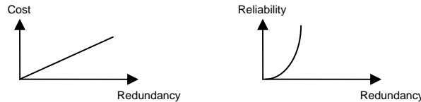
Figure 7-8: The relationship between the cost to establish redundancy, and the reliability resulting from redundancy (Ahlmann, 1992)
