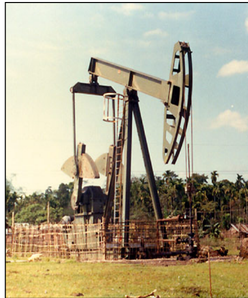
Figure 17. The figure shows field operation a sucker rod pump.
