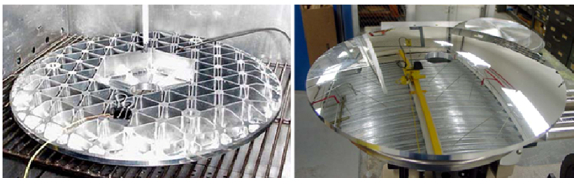
Figure 153. SOFIA secondary-mirror blank (backside on the left and frontside on the right. This mirror vibrates with a frequency of 20 Hz in chopping mode (Erikson, et.al, 2004).
