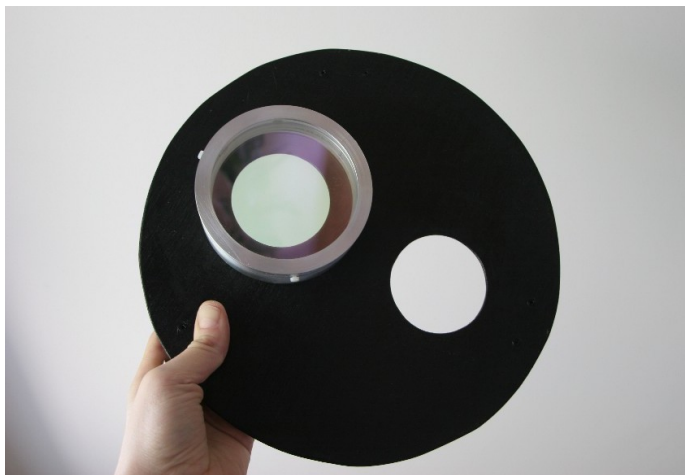
Figure 74. A DIMM aperture plate seen from its front side (Sarazin, ESO).
