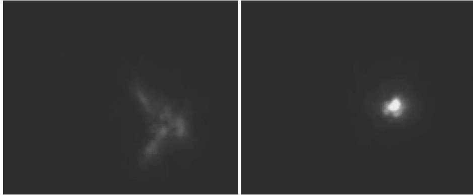
Figure 62. Images of Altair observed with the SCAO system. Left-hand box shows the image with open loop, right-hand box with closed loop.
