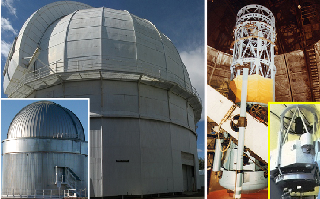
Figure 132. Nordic Optical Telescope and Hooker telescope, both with approximately 2.5 m apertures but with different primary-mirror focal ratios, 2.0 and 5.0, respectively. The two telescopes and their enclosures are compared. In both cases, the same scaling is applied.
