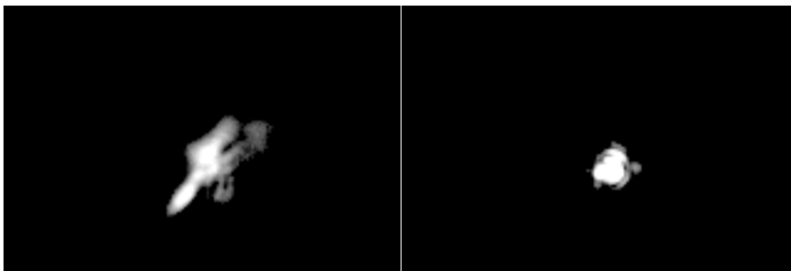
Figure 57. Simulated SCAO corrections of point-source object. Left-hand box shows object without correction, right hand box with correction.
